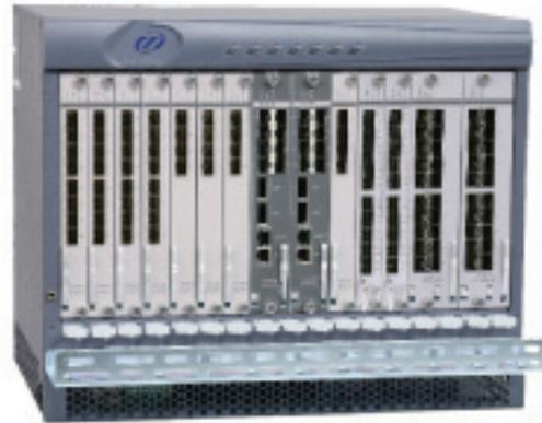
FTTH GPON Services MXK supports G.994.x standards-based GPON to the home with 2.5 Gbps downstream and 1.25 Gbps upstream. MXK offers both 4 or 8 port GPON card that supports 1-64 PON splits per fiber. RF video overlay is supported using a 1550nm wavelength for the RF signal over GPON.
