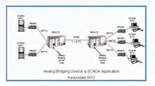
Each bridge can contain up to a maximum of 30 participants. Bridge to Bridge configurations are supported. The Bridge Server card can add as participants 240 DS0's, originating from the shelf or via transport. UP to eighty bridges can be configured, but total DS0 capacity is limited by use of compression and echo cancellation.
