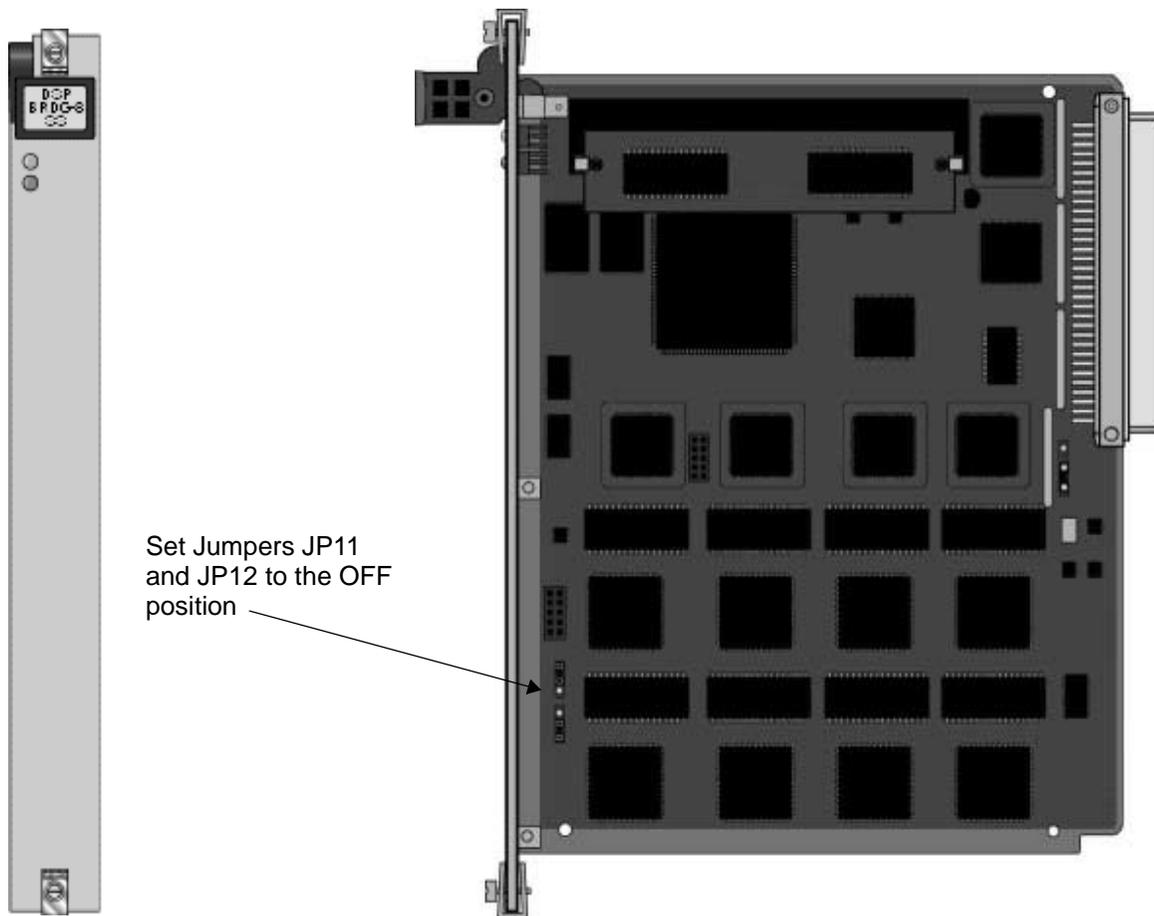
**Figure 9-1. Analog Bridge Server Card Jumper Settings**
