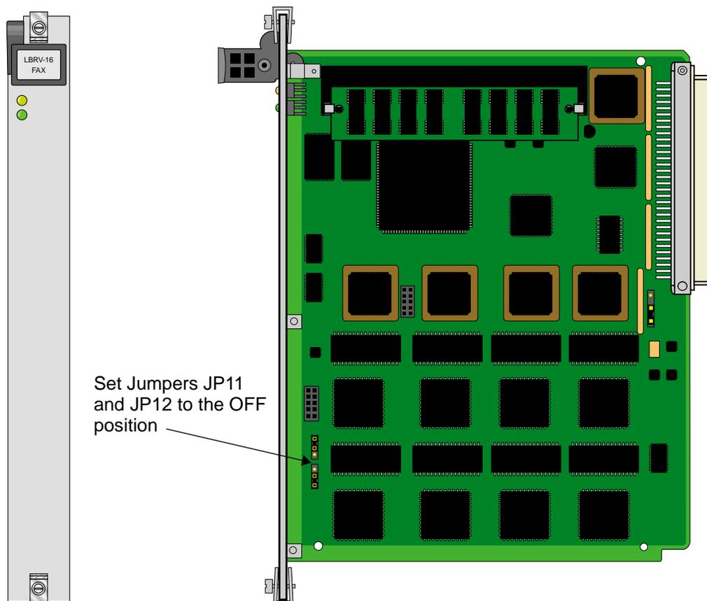
**Figure 7-3.LBRV-16 FAX Card Jumper Settings**
