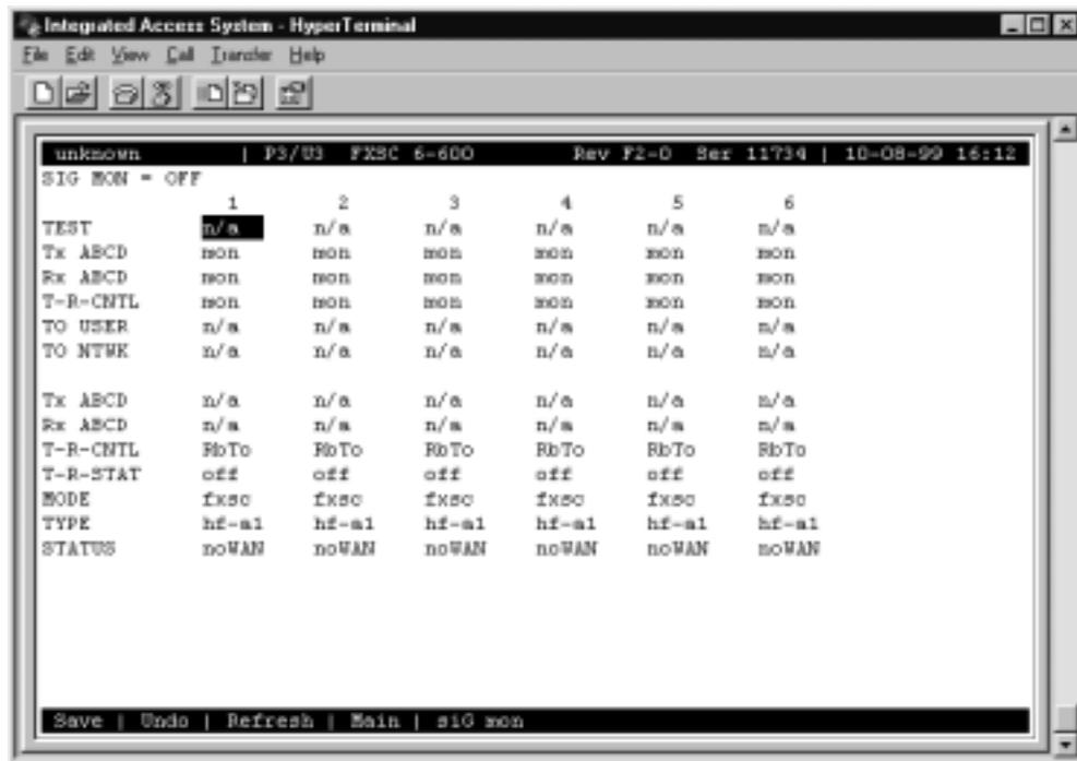
Figure 5-4. Typical FXS Coin Card Test Screen
