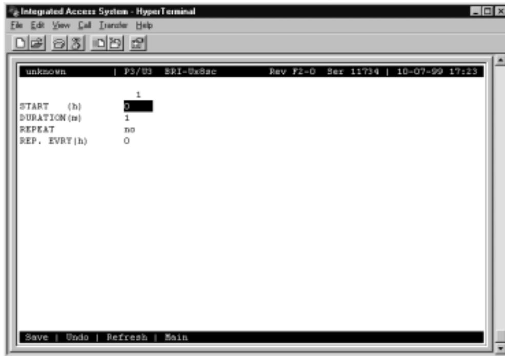
**Figure 8-5. Typical BRI-SC U\*8 Card Sealing Current Screen**
