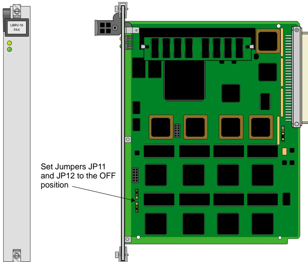
**Figure 7-3.LBRV-16 FAX Card Jumper Settings**
