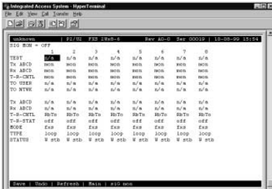
Figure 2-4. Typical FXS Card Test Screen
