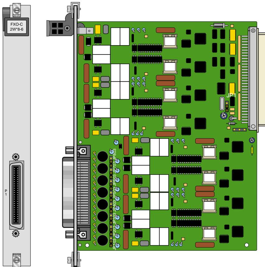
**Figure 6-1. Jumpers Settings for FXO Coin Card**
