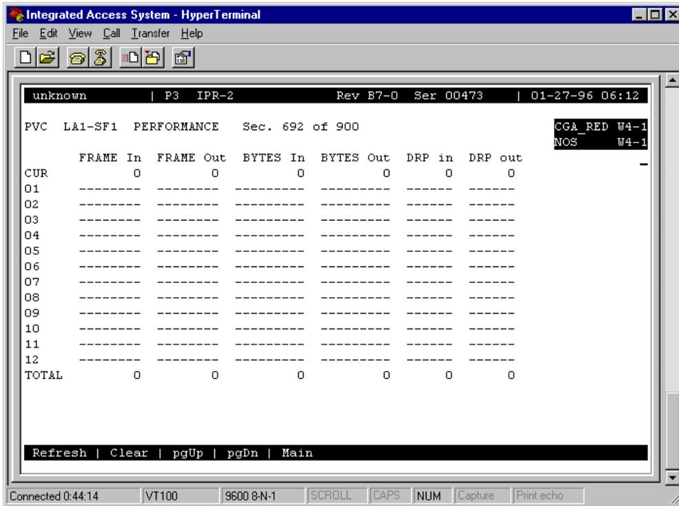
Figure 8-15. IPR 10B2 and 10BT PVC Performance Screen
