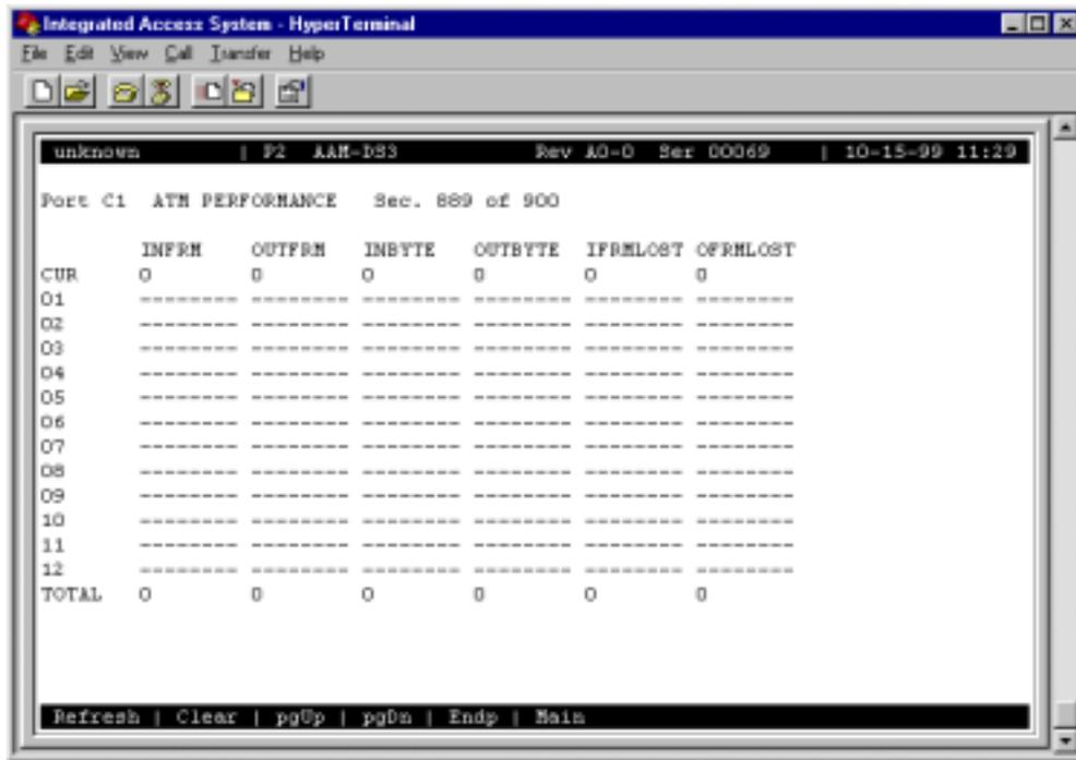
**Figure 4-7. Typical VBR Port Performance Data Screen (ATM)**
