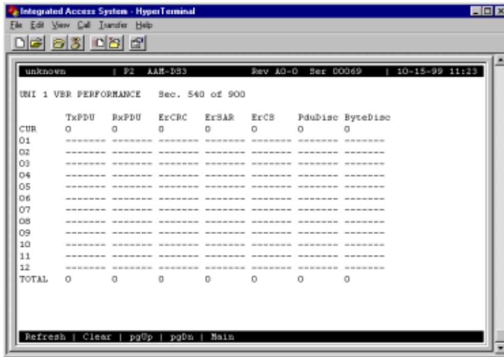
Figure 4-4. Typical UNI VBR Performance Data Screen
