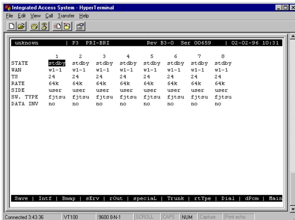
Figure 6-8. D Channel Configuration Screen
