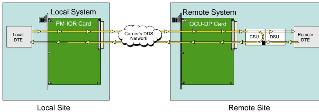
Figure 9-7. Remote CSU Loopback
