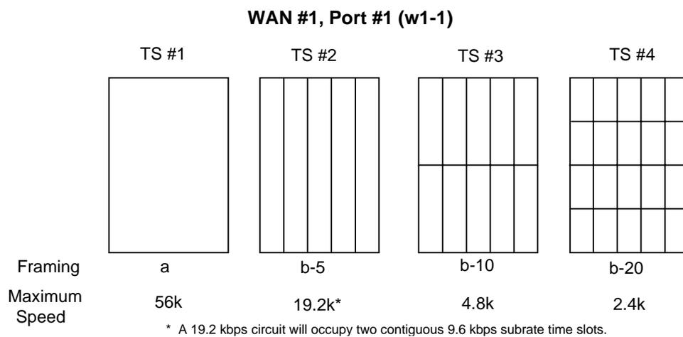
**Figure 4-2. Data Frames, Rates, and Time Slot Assignments**
