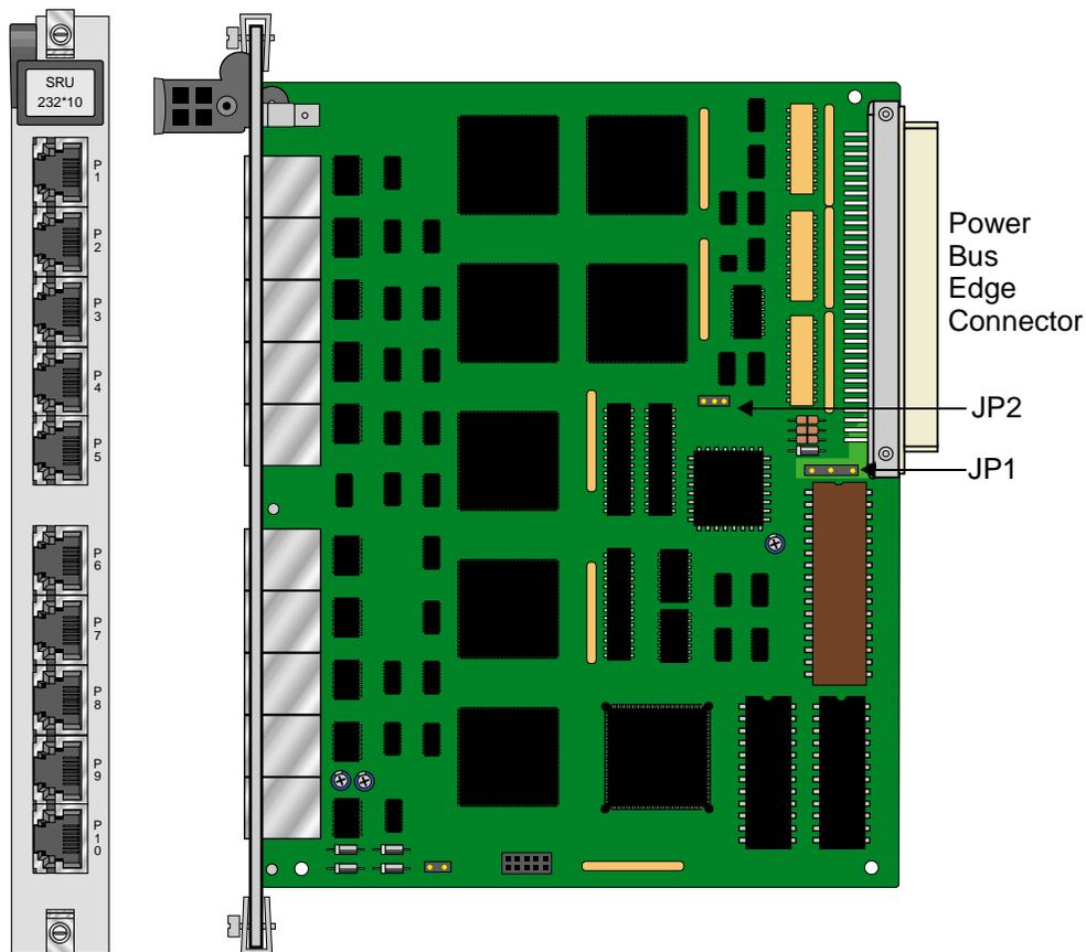
Figure 3-1. SRU 232\*10 Jumper Settings
