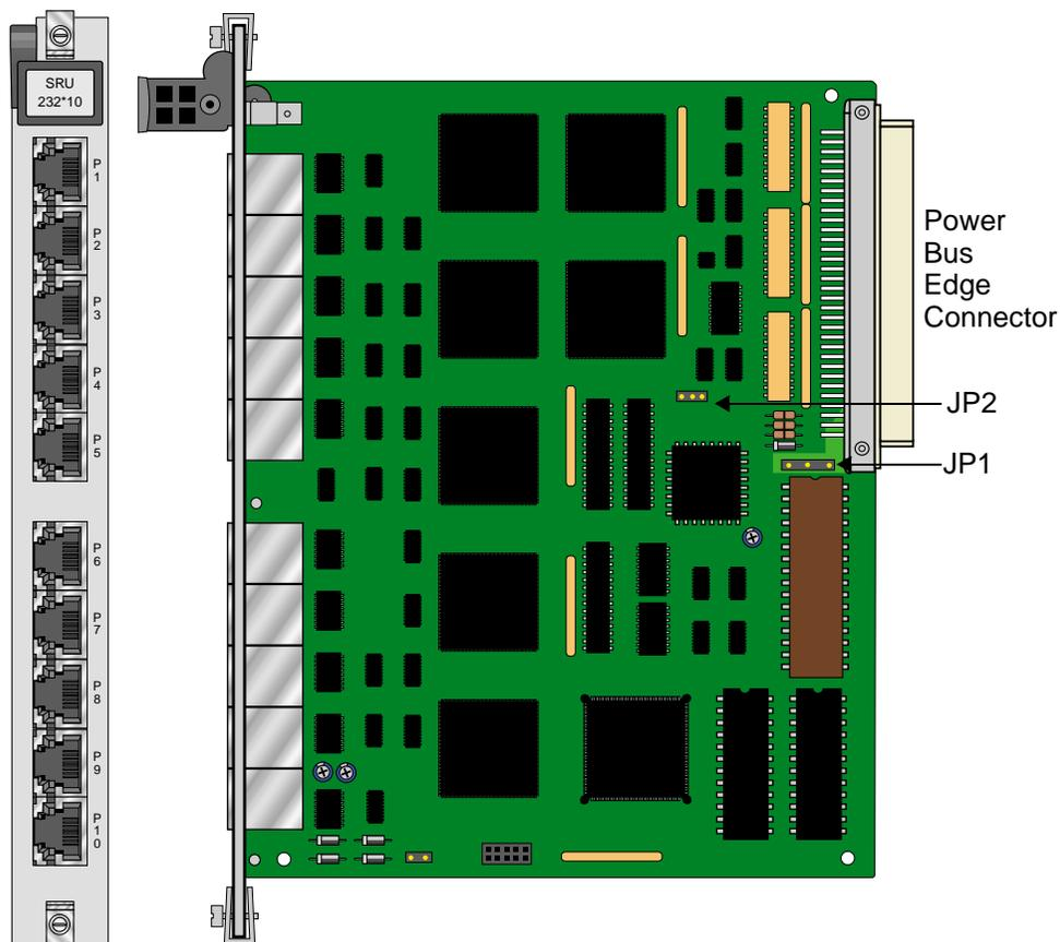
Figure 3-2. SRU 232\*10 C&D Bus Jumper Settings
