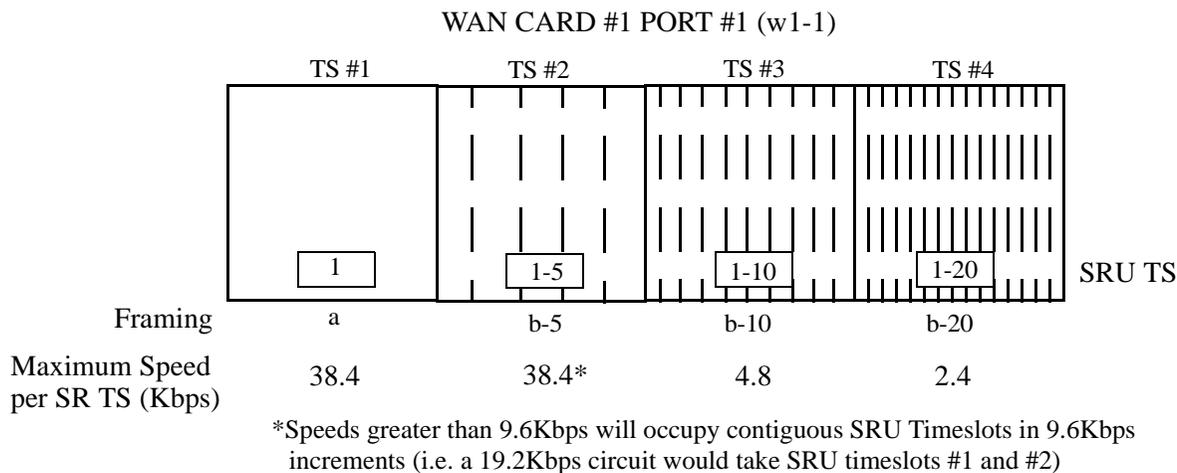
**Figure 3-6. SRU Time Slot Integration**
