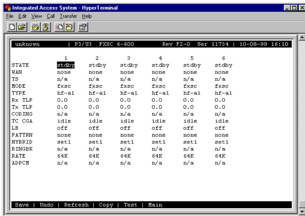
Figure 4-2. Typical FXS Coin Card Main Screen
