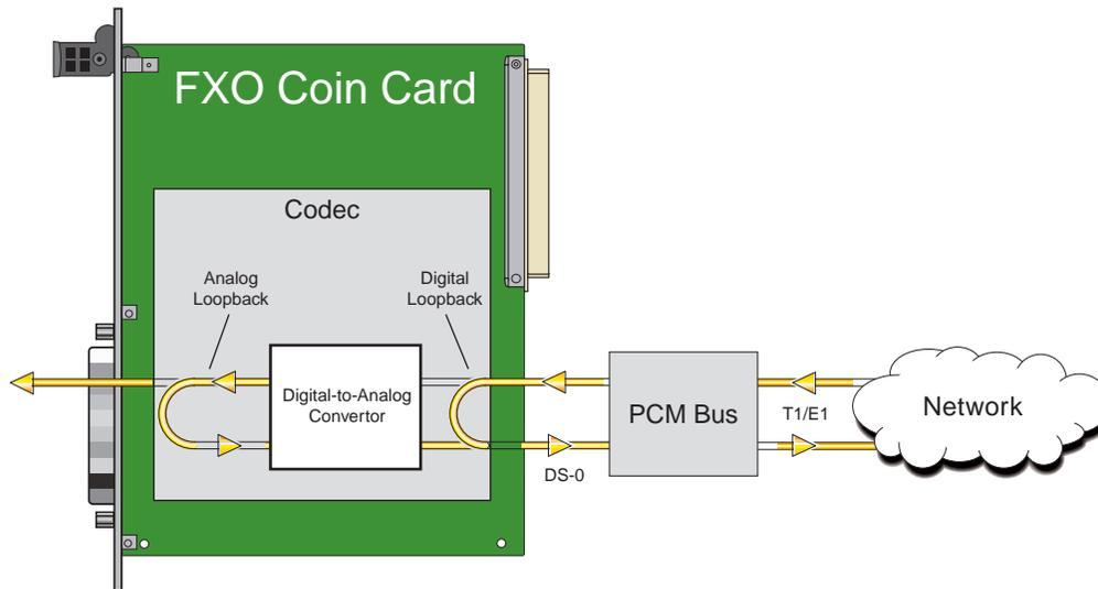
Figure 5-3. FXO Coin Card Loopbacks
