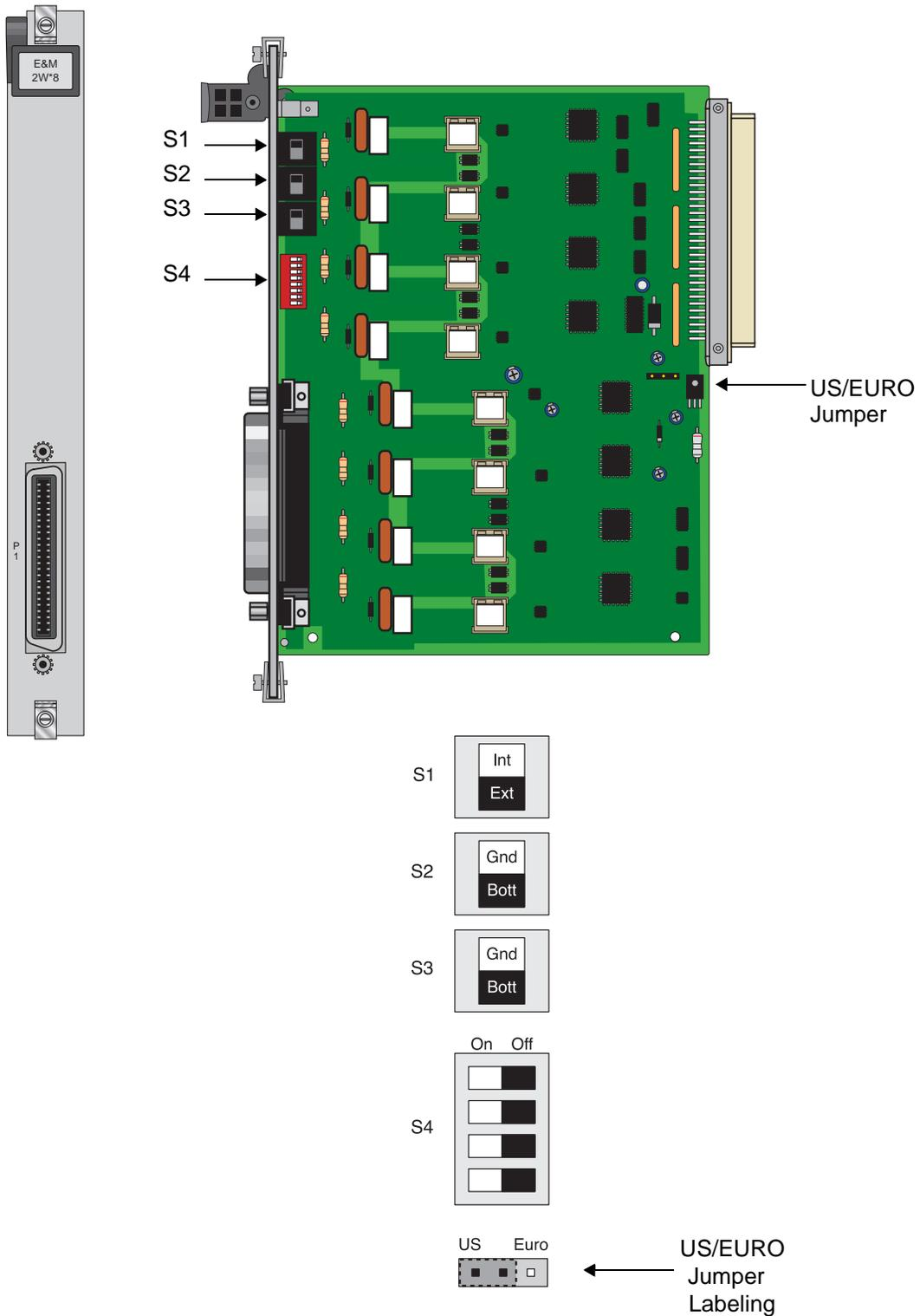
Figure 1-1. Typical E&M Card Switches
