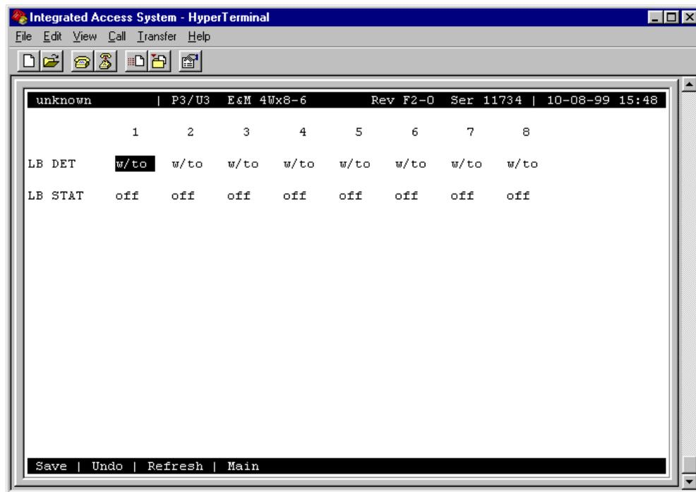
**Figure 1-5. Typical E&M Loopback Screen**
