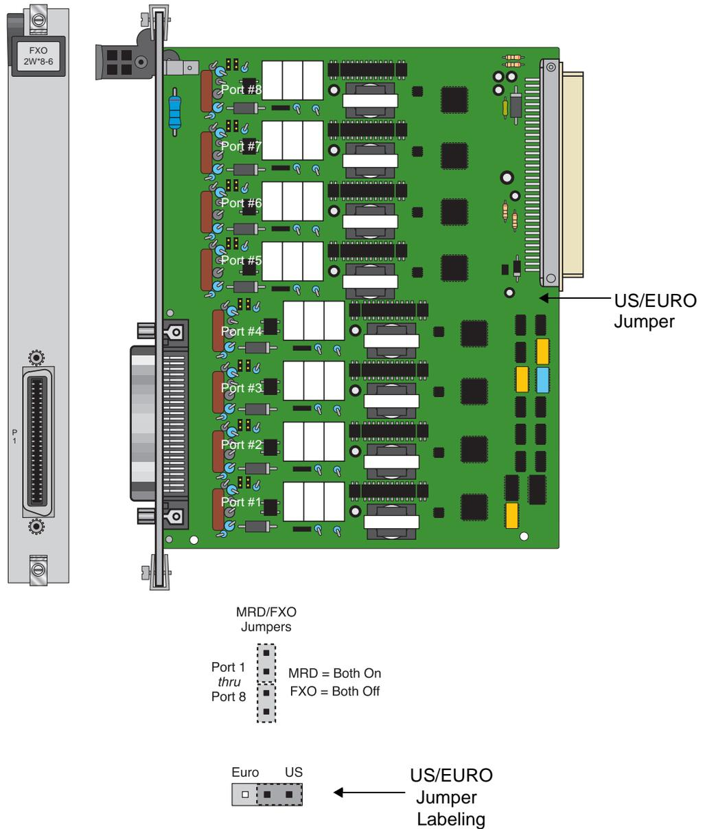
Figure 3-1. FXO 2W\*8-6 Card Jumper Settings
