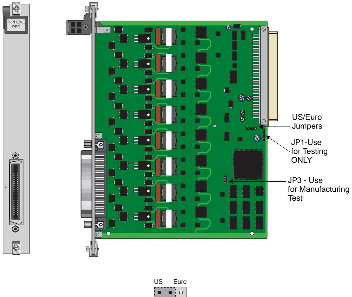
Figure 7-1. P-Phone PPO and PPS Cards Jumper Settings
