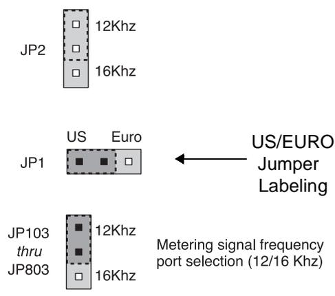
Figure 5-1. Jumpers for MRD Mode
