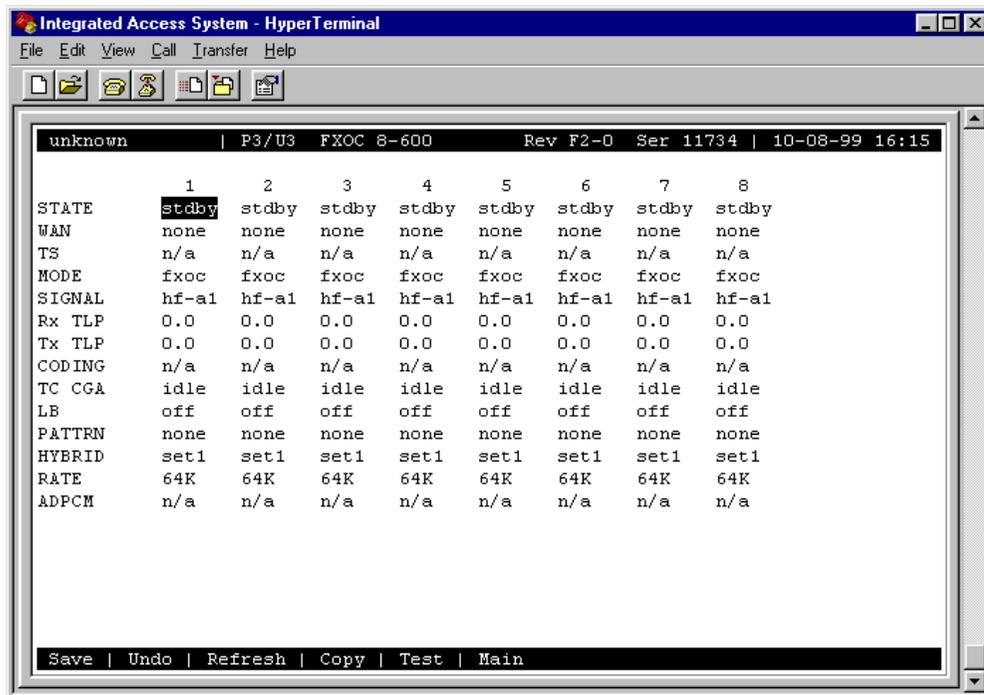
Figure 5-2. Typical FXO Coin Card Main Screen
