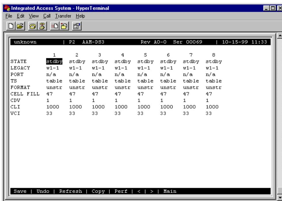
Figure 4-9. Typical CBR Configuration Screen
