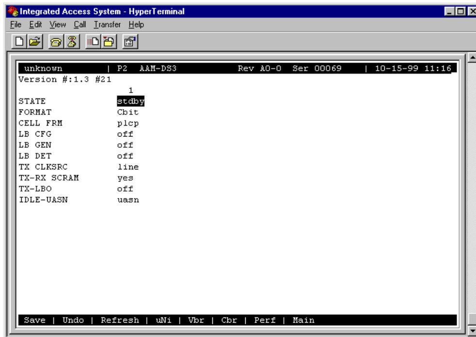
**Figure 4-1. Typical ACS-ATM Card Main Screen (DS3)**
