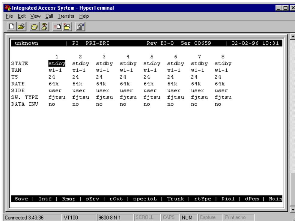
Figure 6-8. D Channel Configuration Screen
