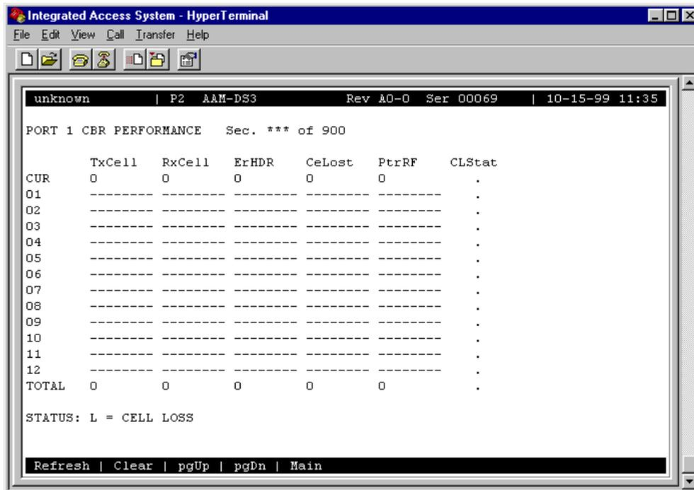
Figure 4-11. Typical CBR Port Performance Data Screen
