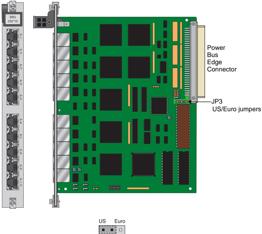
**Figure 2-1. SRU 232\*10 Jumper Settings**
