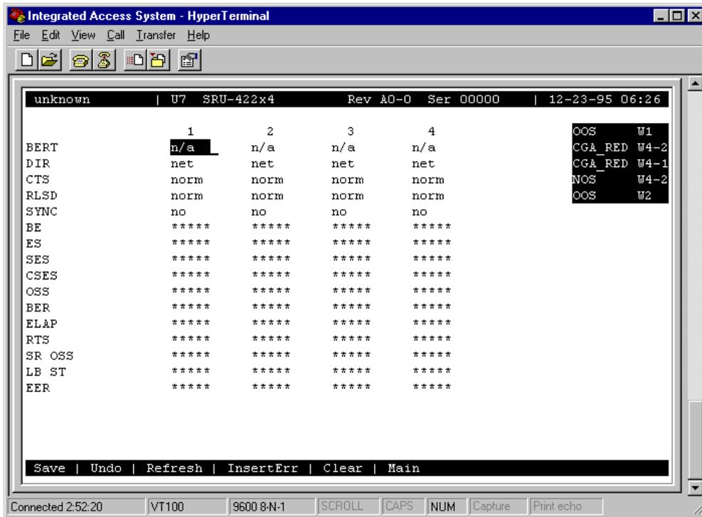
Figure 2-10. Typical SRU Card Test Screen
