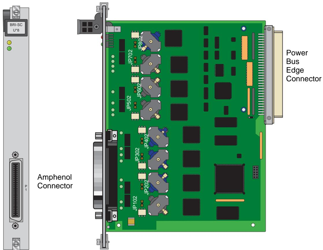
**Figure 7-3. BRI-SC U\*8 Card Sealing Current Jumpers (826170/71)**
