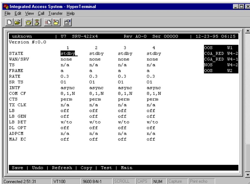
Figure 2-3. Typical SRU Card Main Screen
