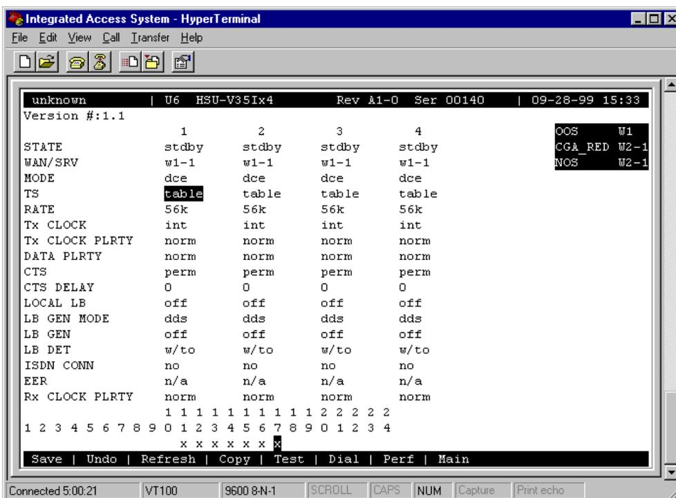
Figure 1-9. Typical HSU Port Time Slot Assignment Screen
