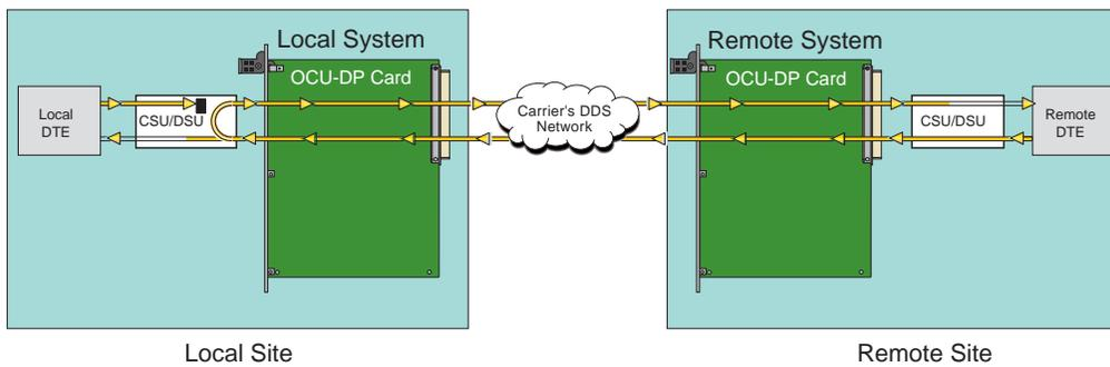
**Figure 3-8. OCU Remote Loopback (csu-u option)**
