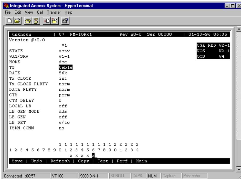
Figure 8-3. Typical PM-IOR Port time slot Assignment Screen
