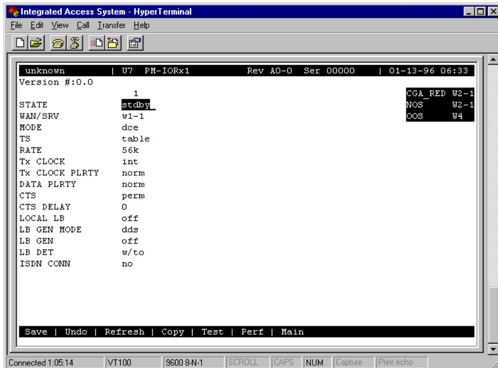
**Figure 8-2. Typical PM-IOR Card Main Screen**
