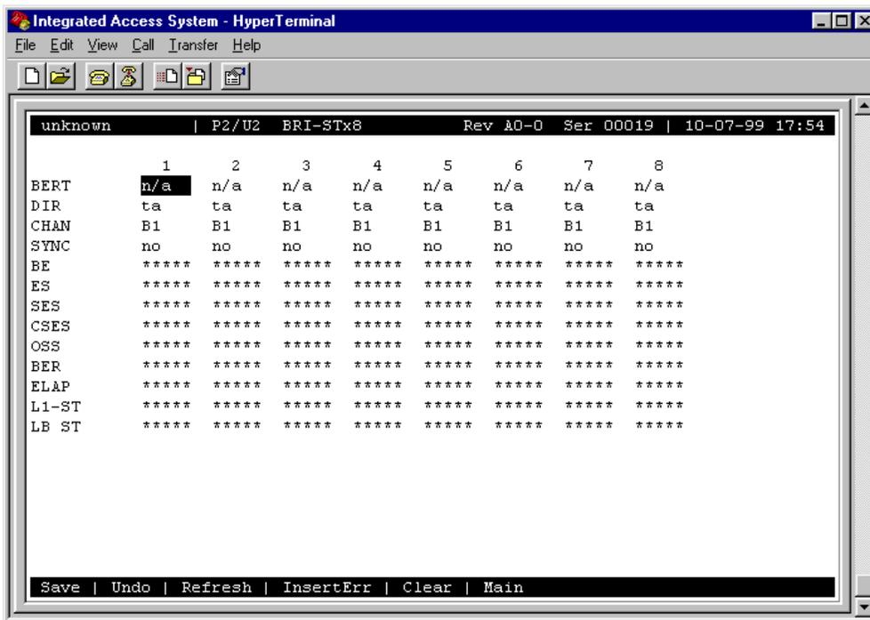
Figure 7-18. Typical BRI-ST\*8 Card Test Screen
