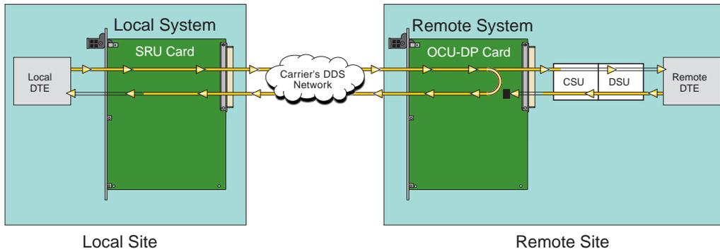
Figure 2-6. Inband Remote SRU Loopback
