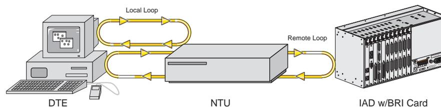
**Figure 7-14. Local and Remote Loopback Testing**
