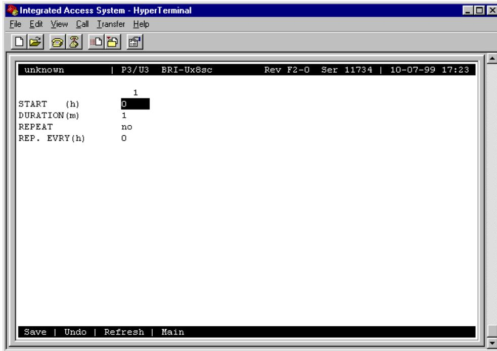
Figure 7-5. Typical BRI-SC U\*8 Card Sealing Current Screen
