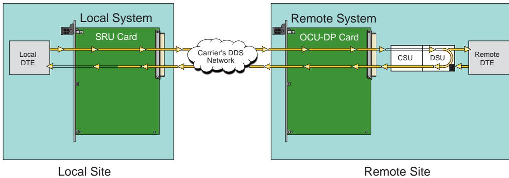
Figure 2-8. Inband Remote DSU Loopback
