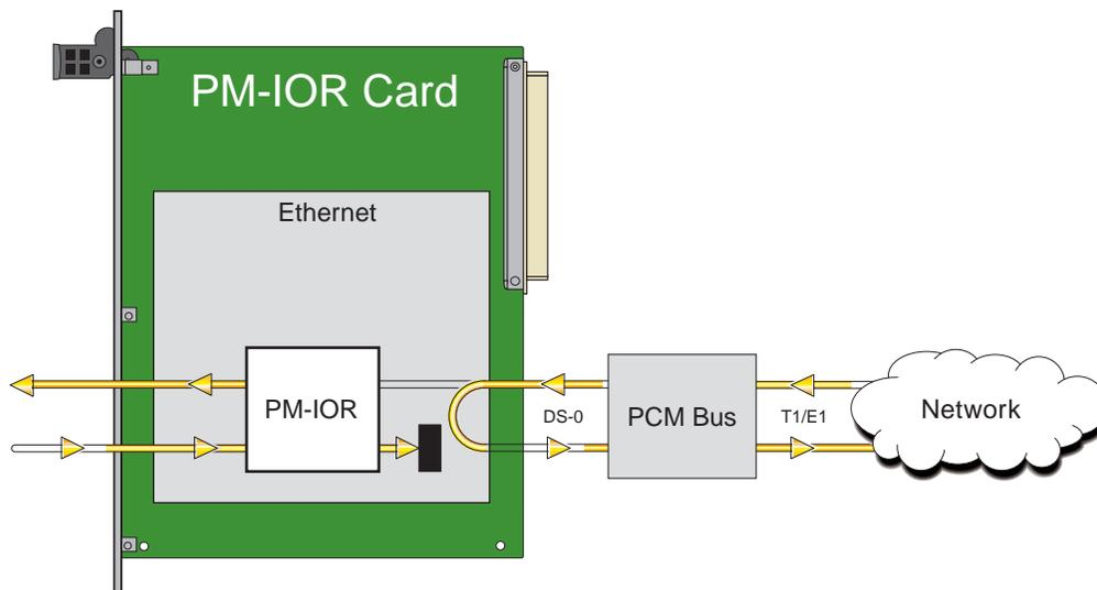
**Figure 8-4. Local DTE Loopback**
