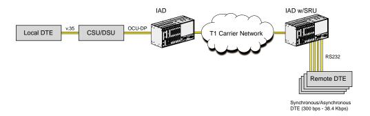
Figure 2-5. IAD with SRU Card Application
