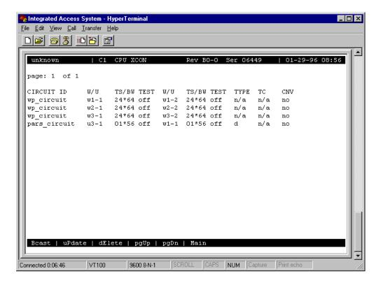
Figure 7-21. System (Main) Cross-Connect Screen in PARS MODE
