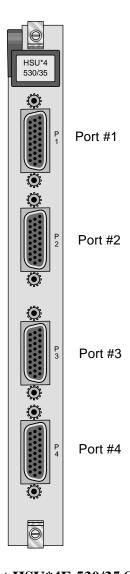
Figure C-31. Four-Port HSU\*4E 530/35 SS Card Jacks (821660)
