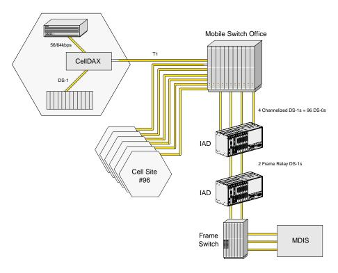
Figure 2-23. Cellular Network Frame Relay Application
