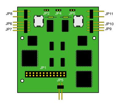
Figure 6-2. Jumper Arrangements for the T1/E1 External Sync Panel
