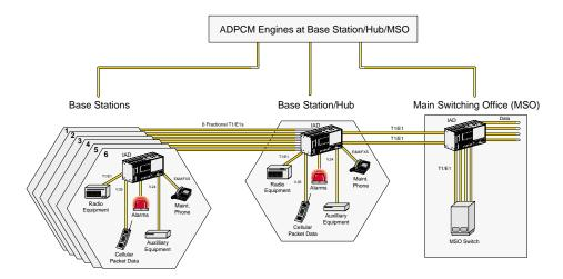
Figure 2-10. IAD in a Wireless Base Station Application
