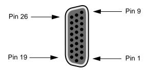
Figure C-26. HSU-AD 530/35 Card Jack Pin Orientation
