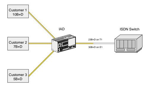
Figure 2-11. Fractional PRI Provisioning using an IAD
