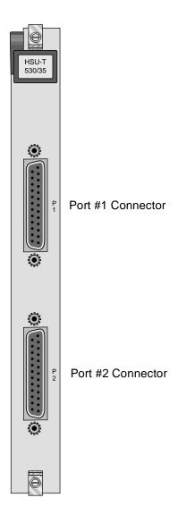
Figure C-28. HSU-T V35 Card Front Panel Connectors (821460)
