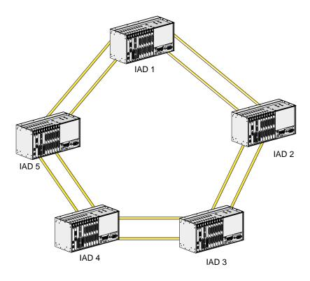
Figure 7-22. Ring Network Traffic Flow
