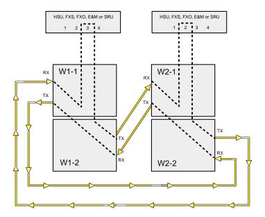
Figure 7-29. PARS Normal Operation Mode (two nodes)
