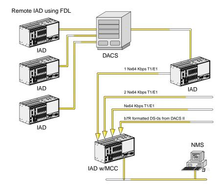
Figure 2-19. MCC Card in a Multilevel Concentration Application
