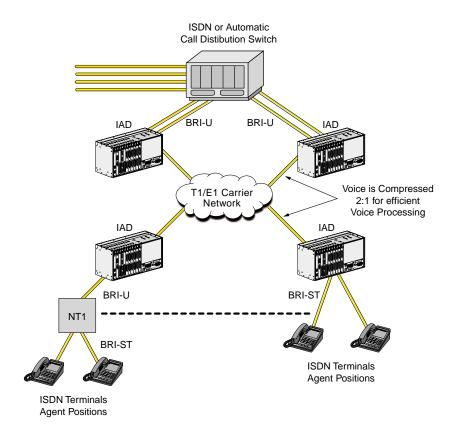
Figure 2-9. IAD in an ISDN-based ACD System
