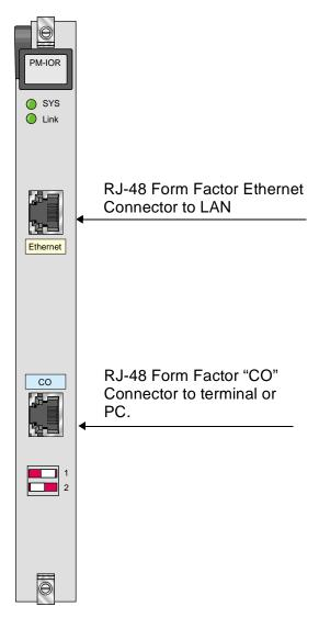
Figure C-43. RJ-48 Form Factor Card Jacks (828060)
