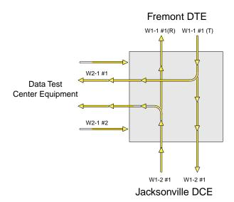
Figure 4-55. Monitor Circuit Diagram
