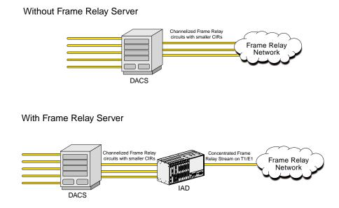
Figure 2-20. IAD using Frame Relay Server Cards
