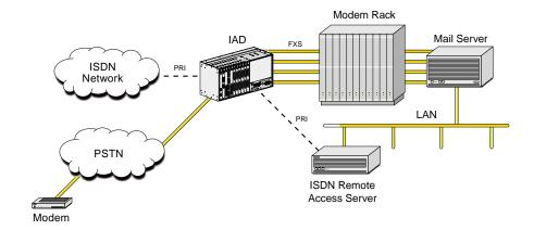
Figure 2-16. PRI to FXS Termination
