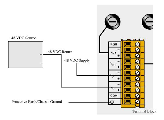
Figure 3-12. DC Terminal Block on Enhanced Chassis with Power Supplies on Top in a DC Environment with one Power Source
