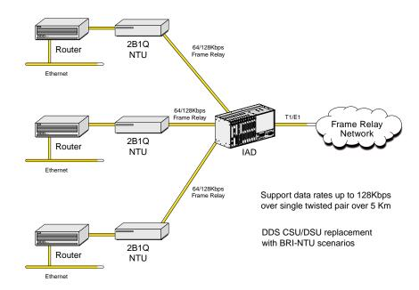
Figure 2-22. IDSL Service Provisioning
