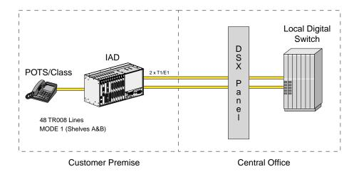
Figure 2-2. IAD using TR008
