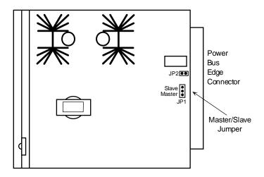
Figure 3-7. 105V Ringing Generator Jumper Setting
