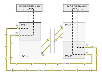
Figure 7-30. PARS Rerouting (two nodes)
