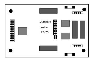
Figure 7-4. DSX/CEPT Module Jumpers (E1 75 Ohm) (81130)
