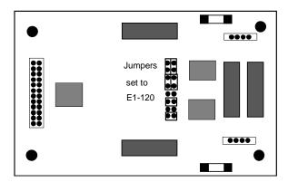
Figure 7-5. DSX/CEPT Module Jumpers (E1 120 Ohm) (81130)
