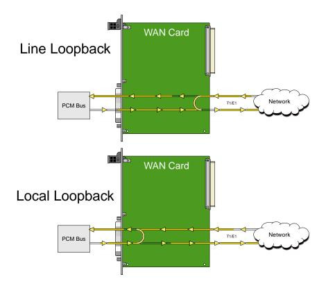
Figure 7-9. Line and Local Loopbacks
