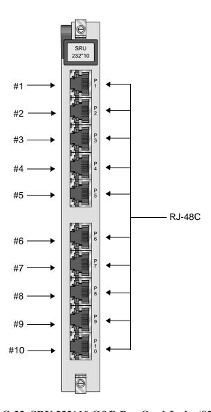
Figure C-33. SRU 232\*10 C&D Bus Card Jacks (822160)
