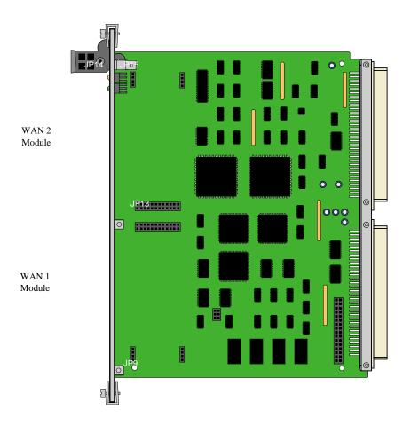
Figure 7-2. Installing DSX/CEPT Modules (8010)
