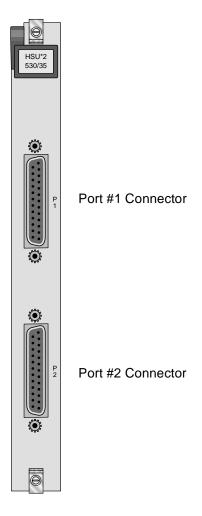
Figure C-21. Two-Port HSU 530/35 Front Panel Connectors (820260)
