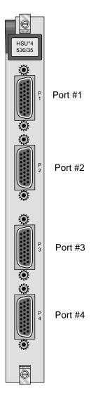
Figure C-30. Four-Port HSU 530/35 Card Jacks (821560)
