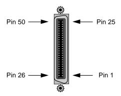
Figure C-56. P-Phone PPO and PPS Card Tip/Ring Connector
