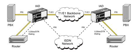
Figure 2-15. IAD using a PRI Server Card for Data Backup
