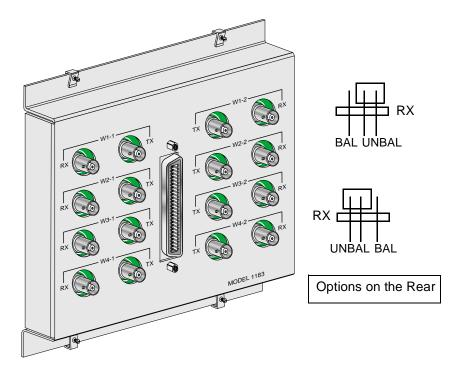
Figure 7-6. E1 Interface Adapter Panel (118320 or 1184)
