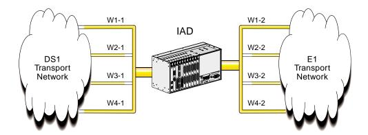
Figure 2-3. IAD using T1/E1 Conversion
