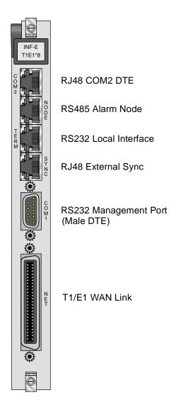
Figure C-1. INF-E Card Connectors (892260)
