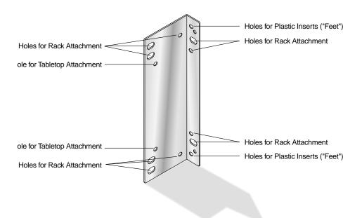
Figure 3-2. Mounting Bracket Holes
