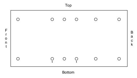
Figure 3-4. Two-Sided Chassis Mounting Holes
