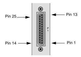
Figure C-22. Two-Port HSU 530/35 Jack Pin Orientation
