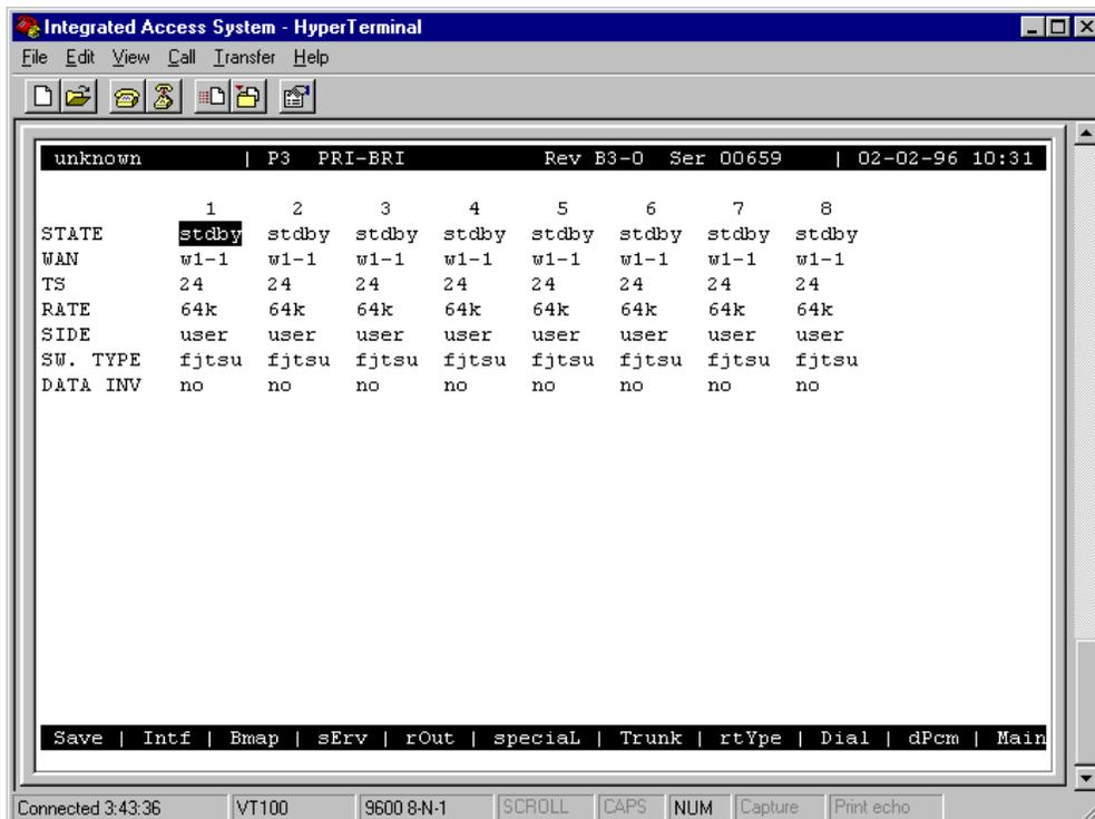
Figure 4-8. D Channel Configuration Screen
