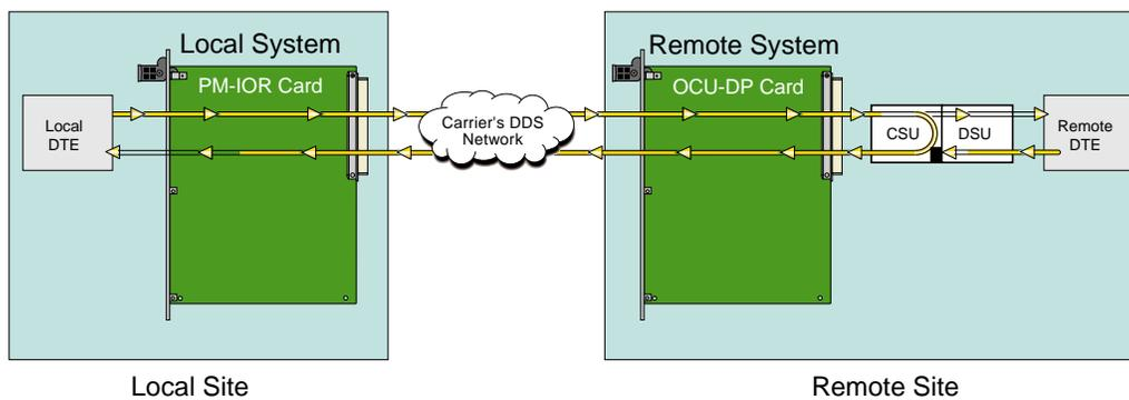
Figure 6-8. Remote DSU Loopback
