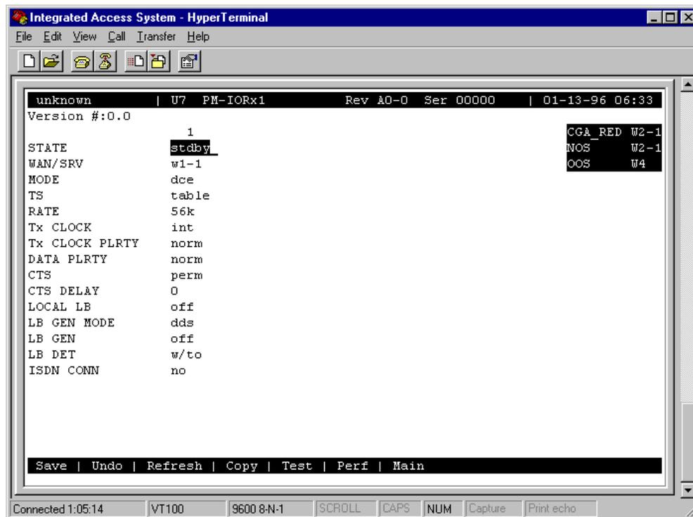
**Figure 6-2. Typical PM-IOR Card Main Screen**
