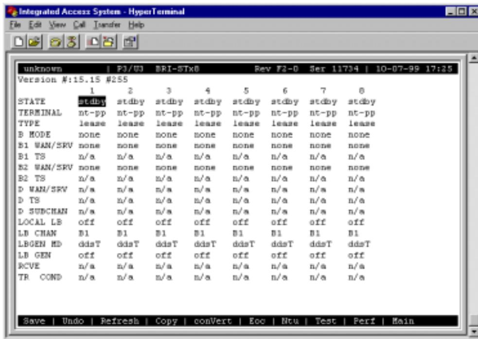
Figure 5-7. Typical BRI-ST\*8 Card Main Screen
