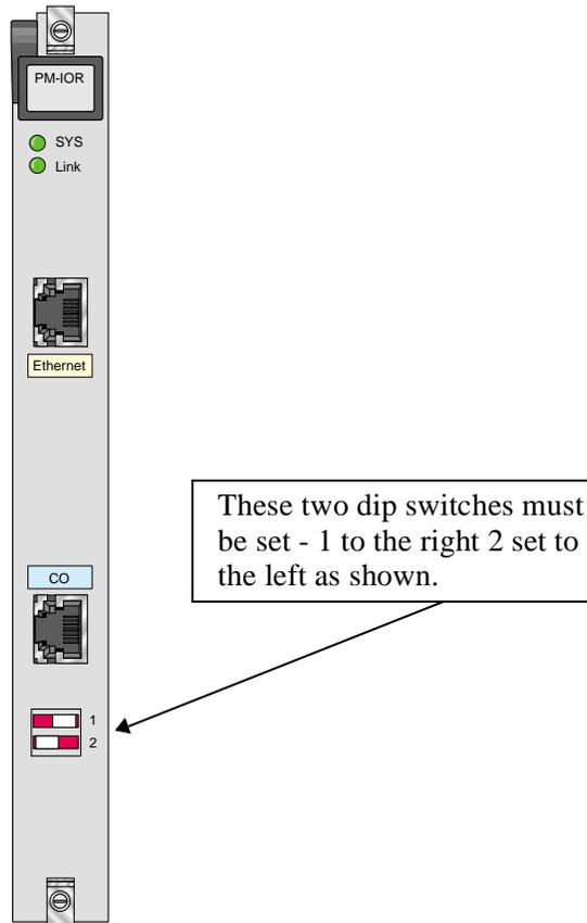
**Figure 6-1. PM-IOR Card Dip-switch settings (828060)**
