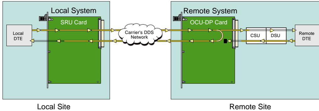
Figure 2-6. Inband Remote SRU Loopback
