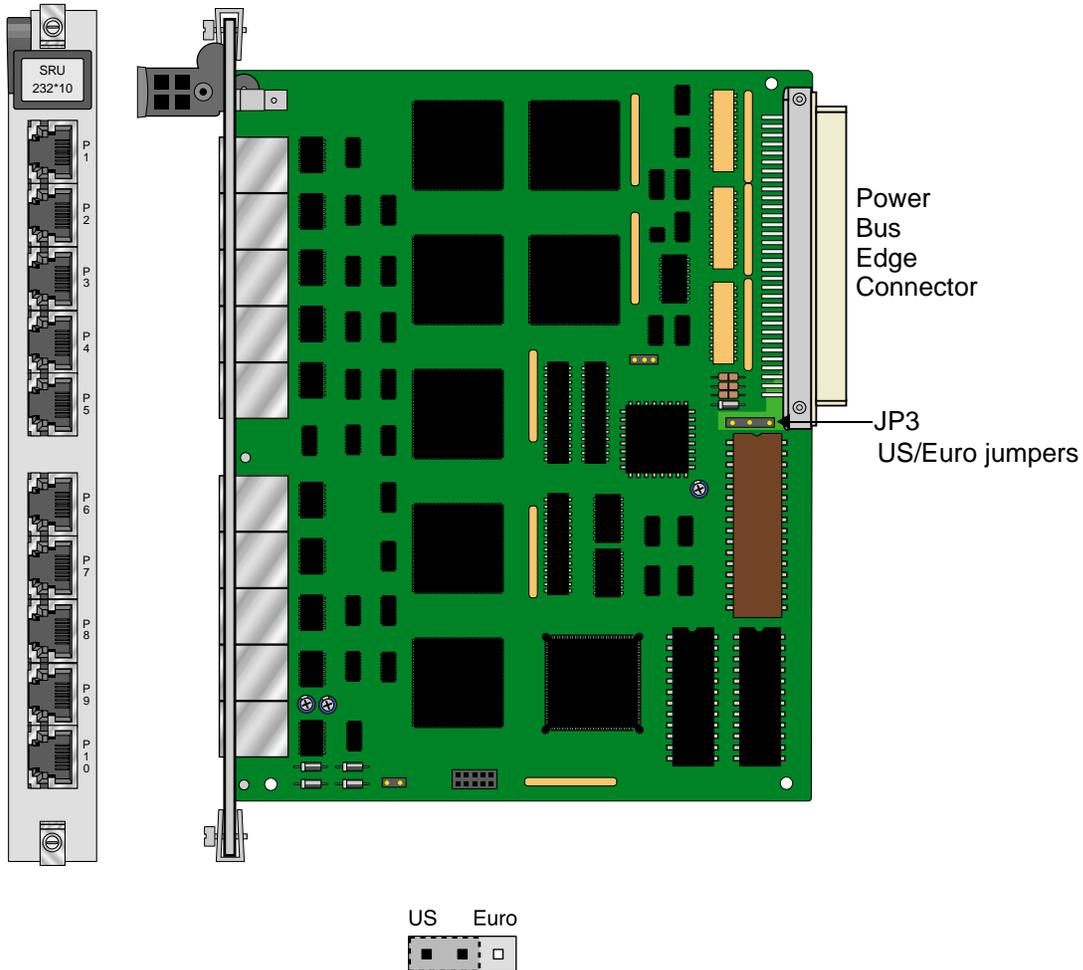
**Figure 2-1. SRU 232\*10 Jumper Settings**
