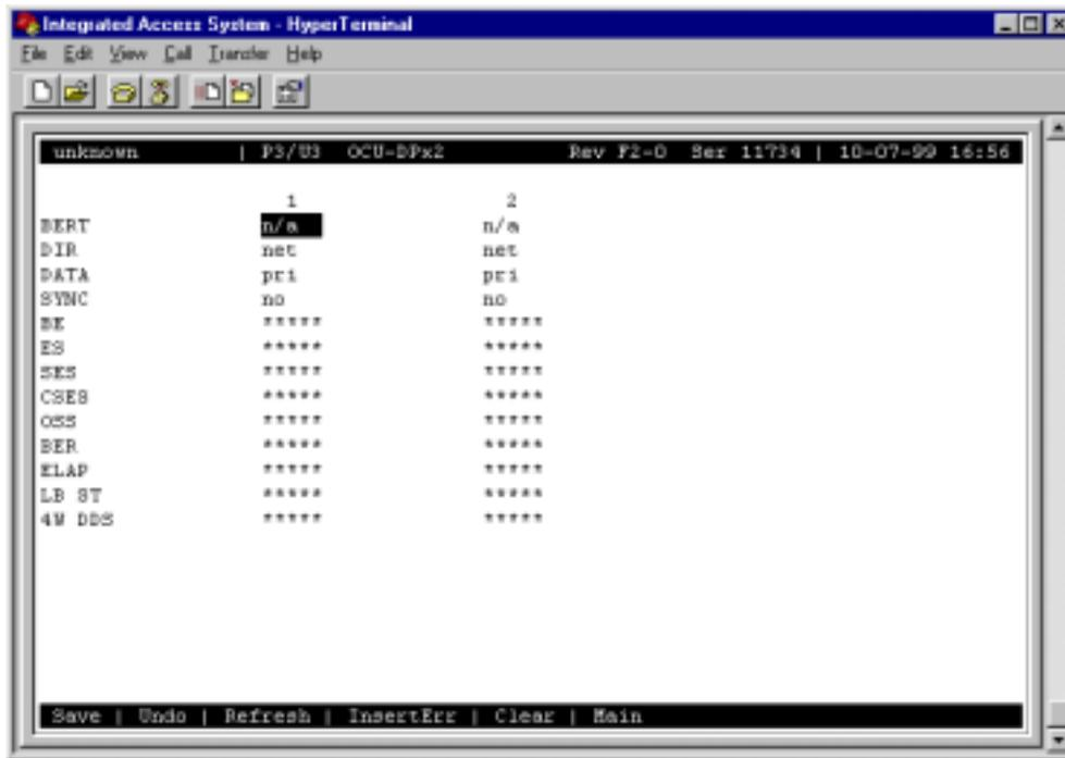
**Figure 3-10. Typical OCU-DP Card Test Screen**
