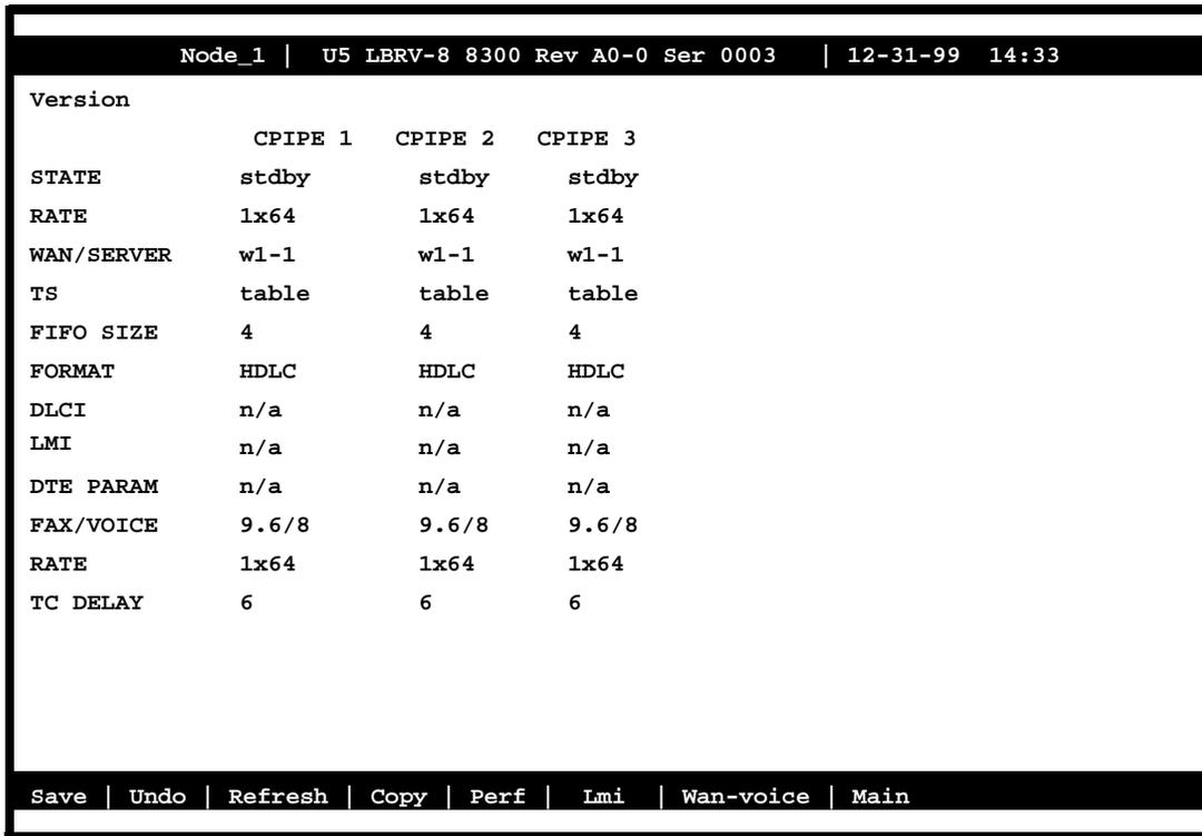
**Figure 6-1. Low Bit Rate Voice Card Main Configuration Screen**
