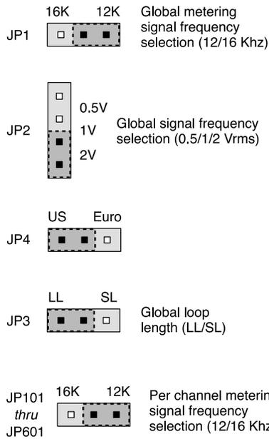
Figure 4-1. Jumper Settings for FXS Coin Card
