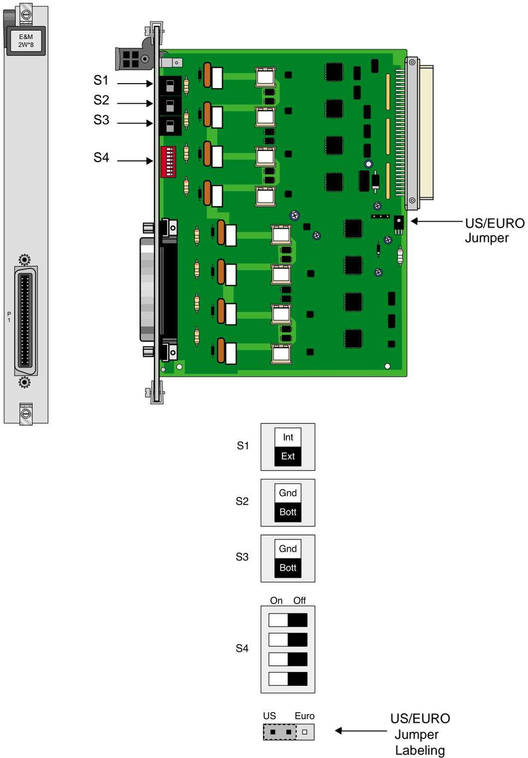
Figure 1-1. Typical E&M Card Switches
