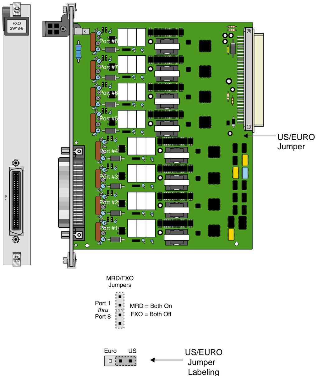
Figure 3-1. FXO 2W\*8-6 Card Jumper Settings
