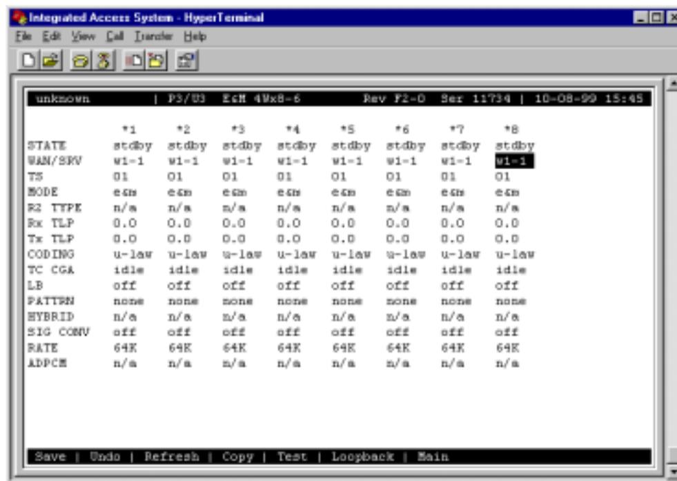
Figure 1-5. E&M Card Main Screen with Loopback
