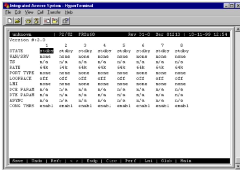
**Figure 2-2. Typical ACS-FRS Card Main Screen (numbered ports)**
