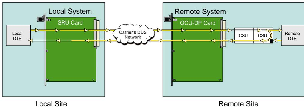
Figure 2-8. Inband Remote DSU Loopback
