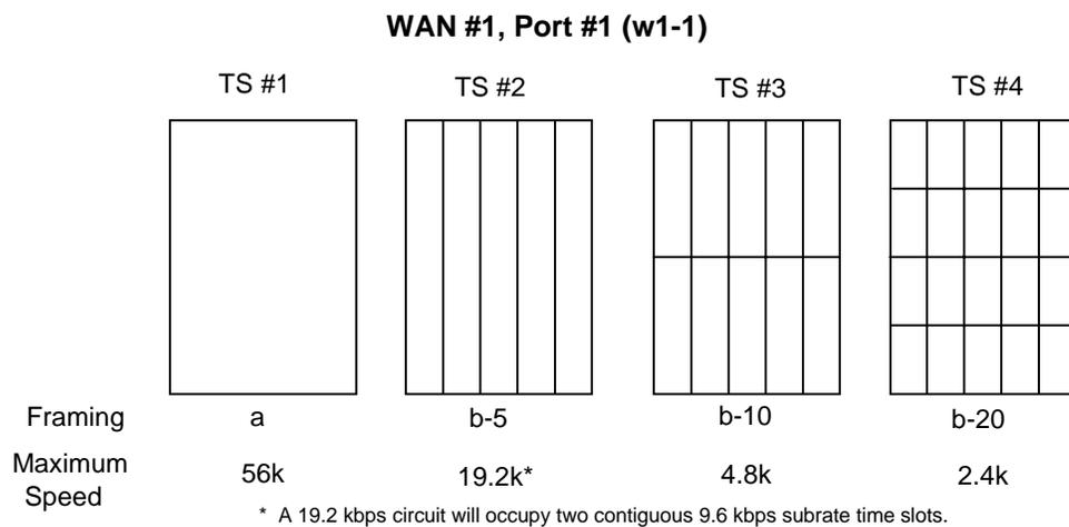
**Figure 3-2. Data Frames, Rates, and Time Slot Assignments**
