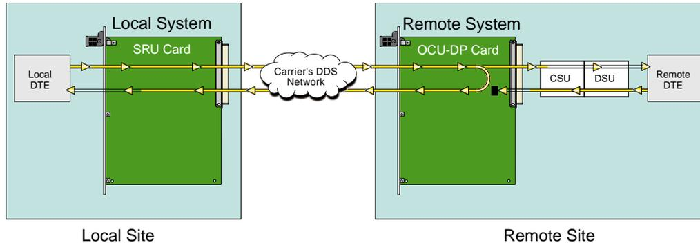
Figure 2-6. Inband Remote SRU Loopback
