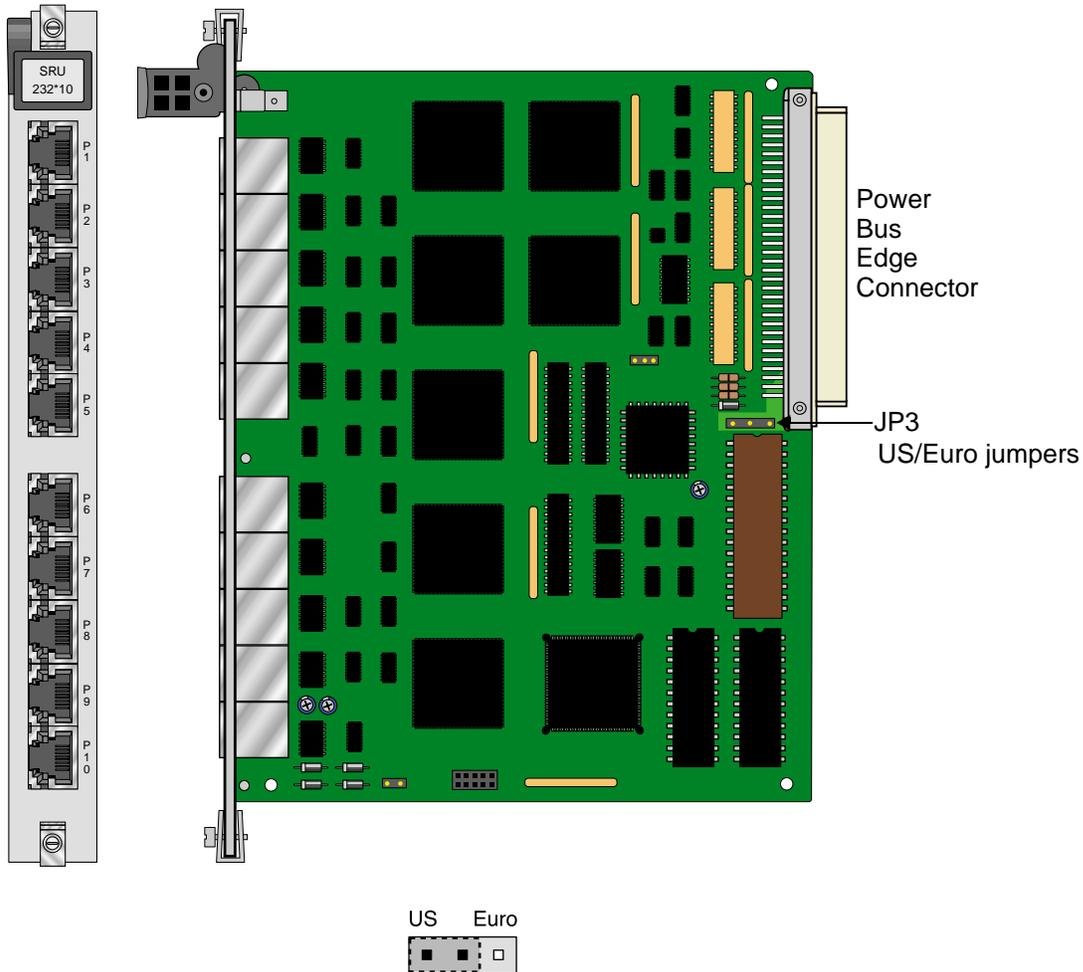
**Figure 2-1. SRU 232\*10 Jumper Settings**
