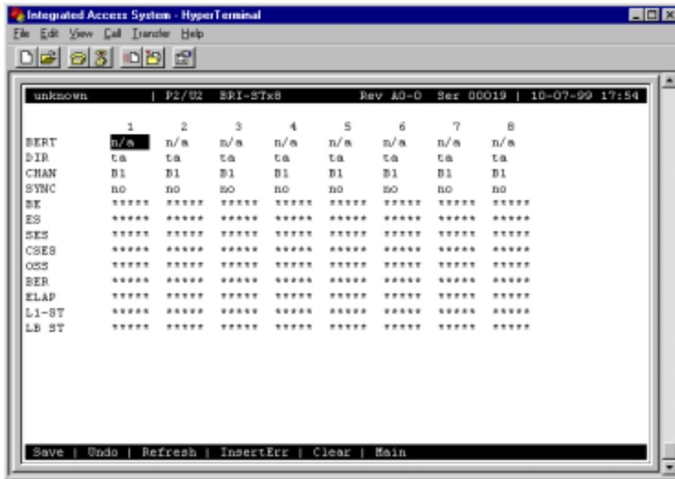
Figure 7-18. Typical BRI-ST\*8 Card Test Screen
