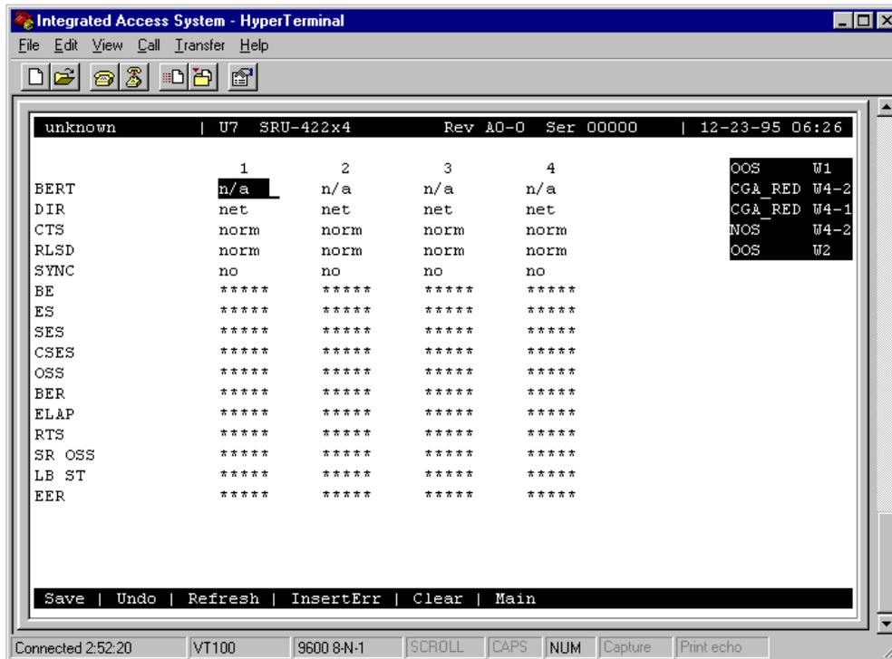
**Figure 2-10. Typical SRU Card Test Screen**
