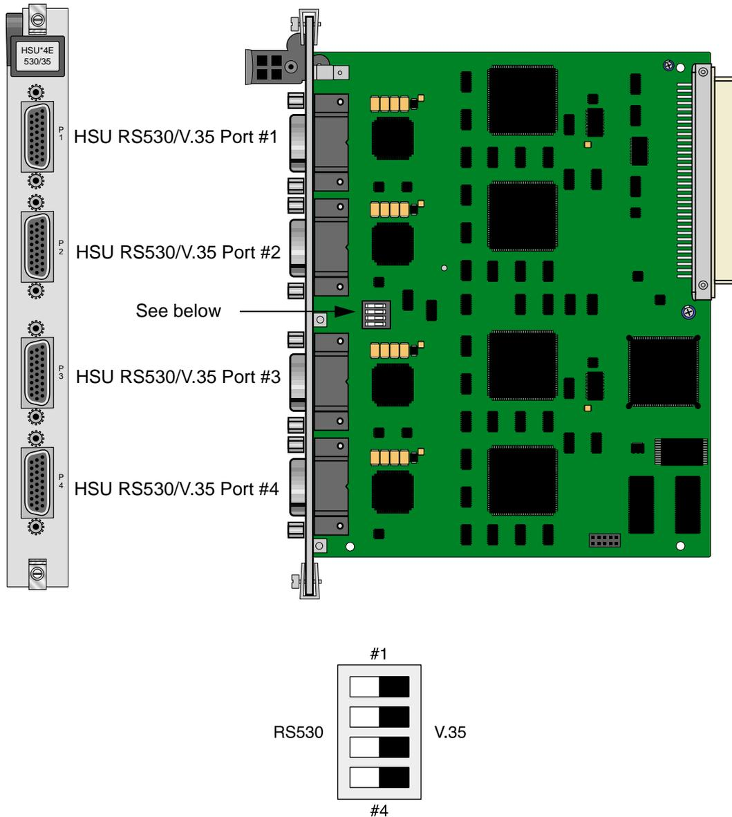
**Figure 1-5. Four-Port HSU\*4E 530/35 SS Card Switches**
