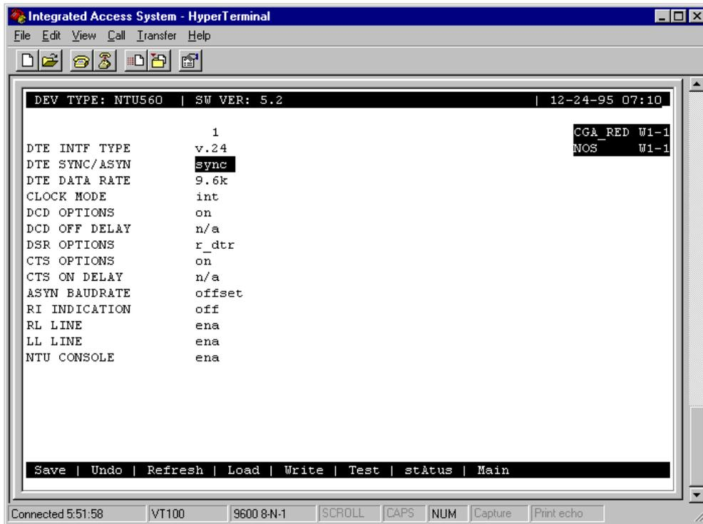
Figure 7-13. Remote NTU Configuration Screen (2560/2561 or 2200E/2201E)
