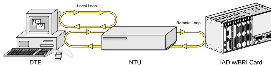
**Figure 7-14. Local and Remote Loopback Testing**
