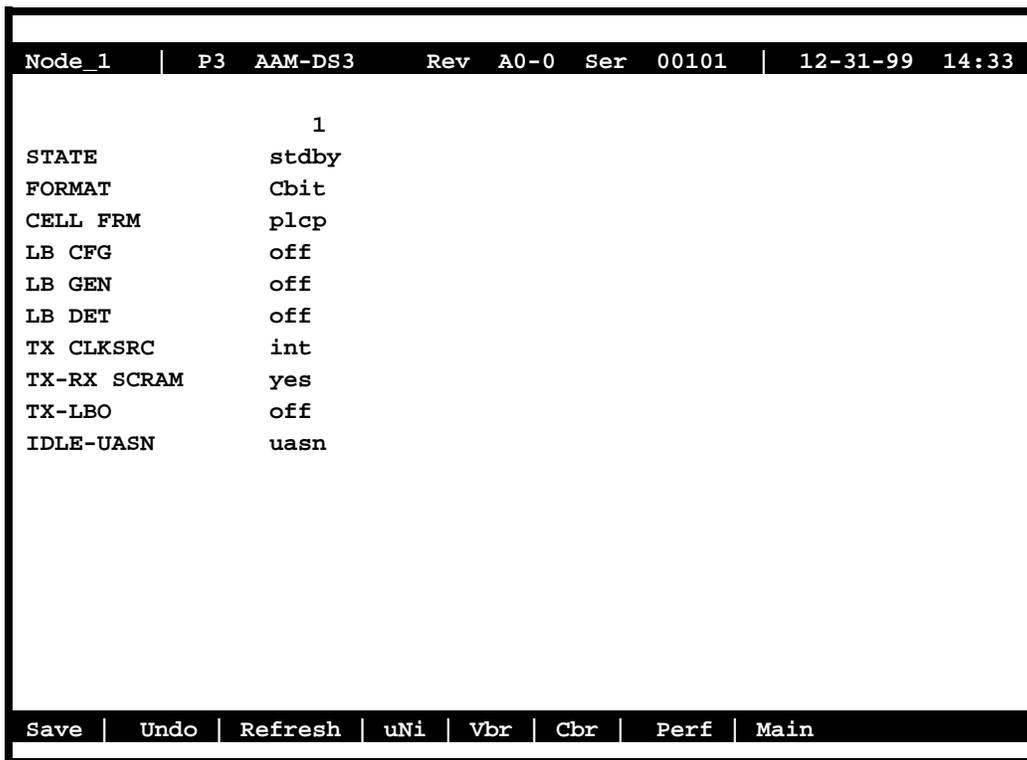
**Figure 4-2. Typical ACS-ATM Card Main Screen (DS3)**
