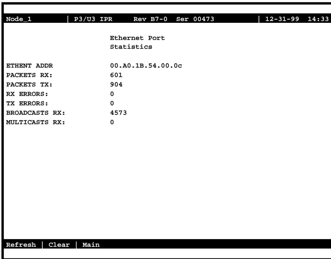
Figure 8-12. Typical Ethernet Performance Screen
