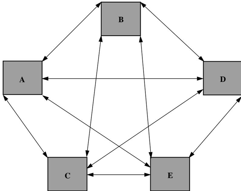
**Figure 8-6. Fully Meshed Frame Relay Network with Full Connectivity**
