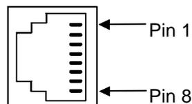
**Figure 4-1. ATM LAN Interface Connector Pin Assignment.**
