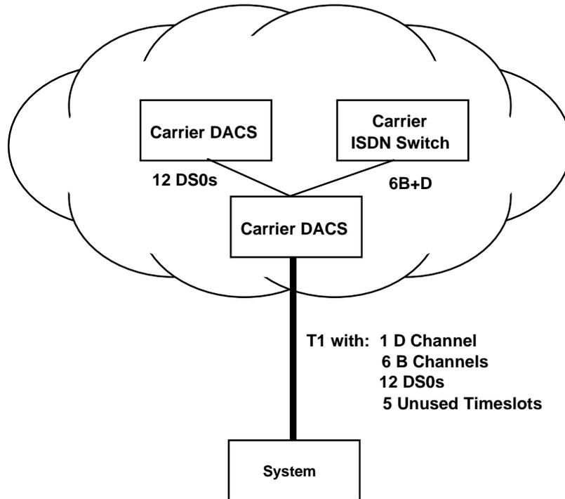
**Figure 6-2. DS0s and B Channels on the Same Facility**
