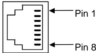
**Figure 8-1. IPR Card Ethernet Port Jack**
