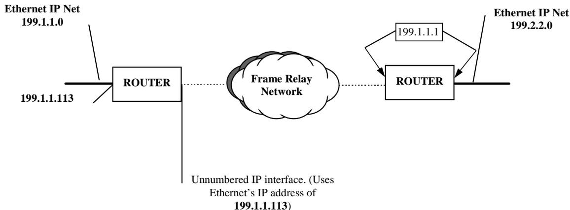
Figure 8-9. Unnumbered Frame Relay IP Interface
