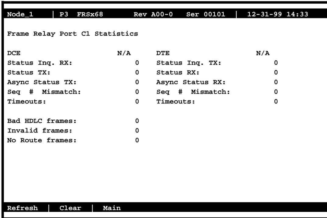
Figure 2-9. Typical LMI Data Screen
