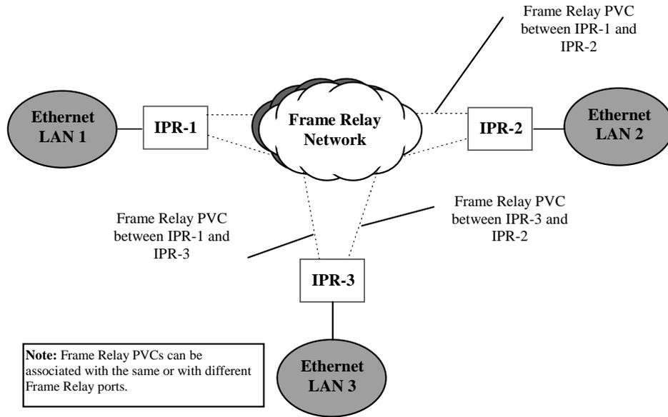
Figure 8-2. IPR Card Connected to IP LANs through Frame Relay Network
