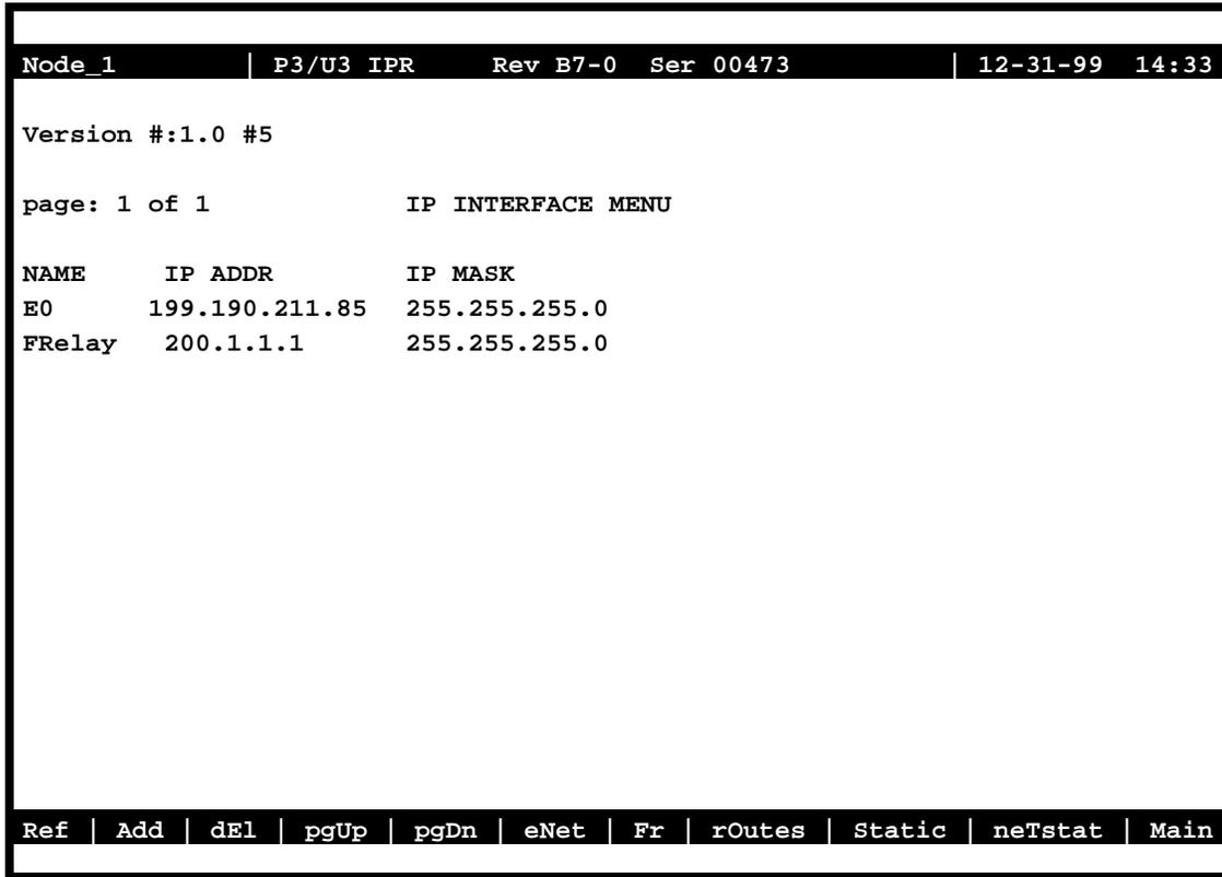
Figure 8-10. IP Interface Main Screen
