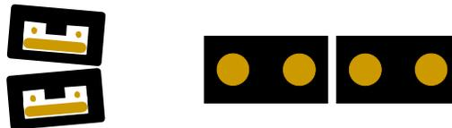
Figure 1-6. Jumper Installation for Active Mode
