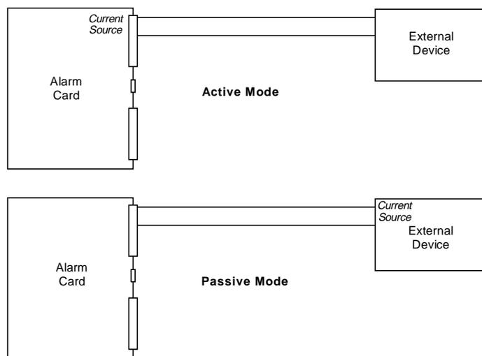
**Figure 1-4. Active and Passive Alarm Sensor Modes**
