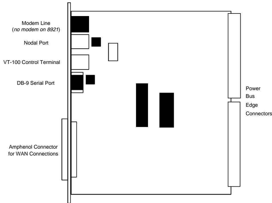
**Figure 5-9. Component Layout for the INF+M T1E1\*8 Interface Card**
