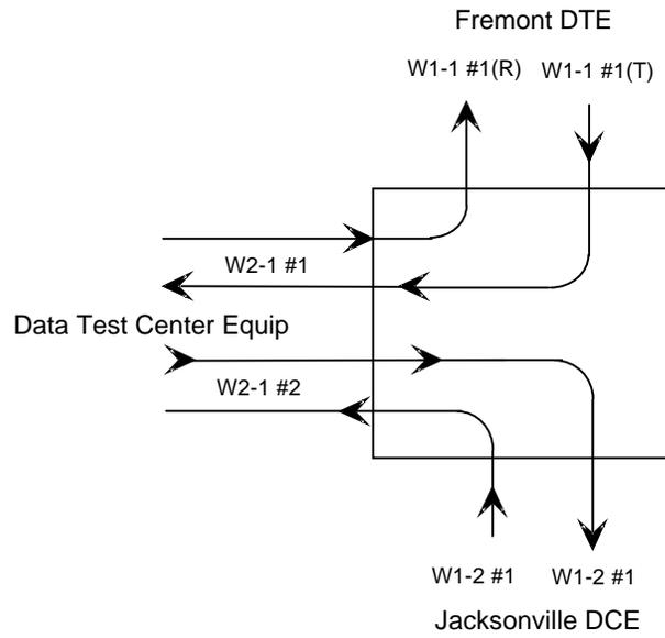
Figure 3-59. Split Circuit Diagram
