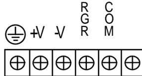
**Figure 2-12. Chassis External Power Connector (rev. C1 +)**
