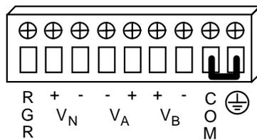
**Figure 2-9. Ground Connections (Front-Loading Chassis with Power Supplies on Side)**
