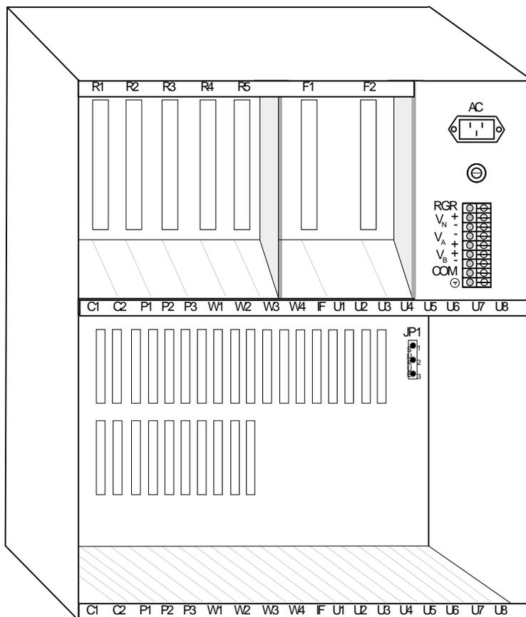
Figure 1-5. Front-Loading Chassis with Power Supplies on Top
