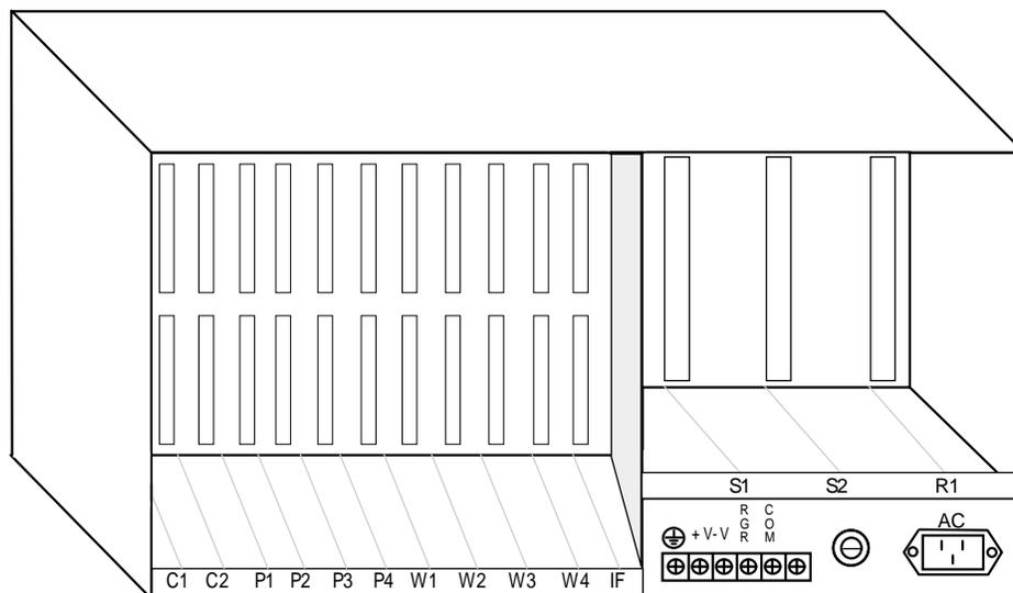
**Figure 1-1. Front-Loading Chassis (four-digit) with Power Supplies on the Side**
