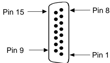
**Figure C-27. HSU-AD 530/35 Card RS-366 Jack Pin Orientation**
