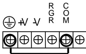
**Figure 2-13. Chassis Ground Connections**
