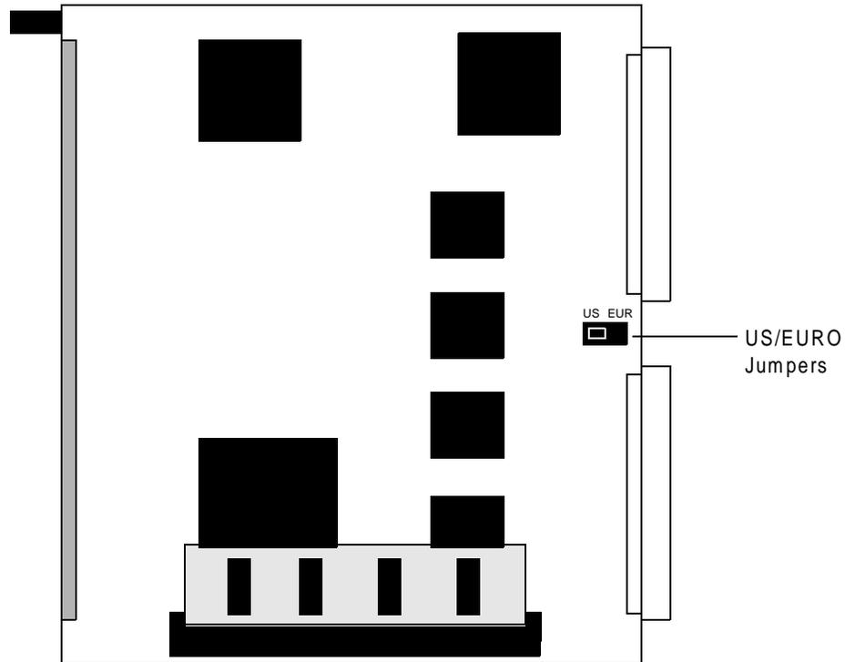
**Figure 4-1. CPU XCON US/EURO Jumper Settings**
