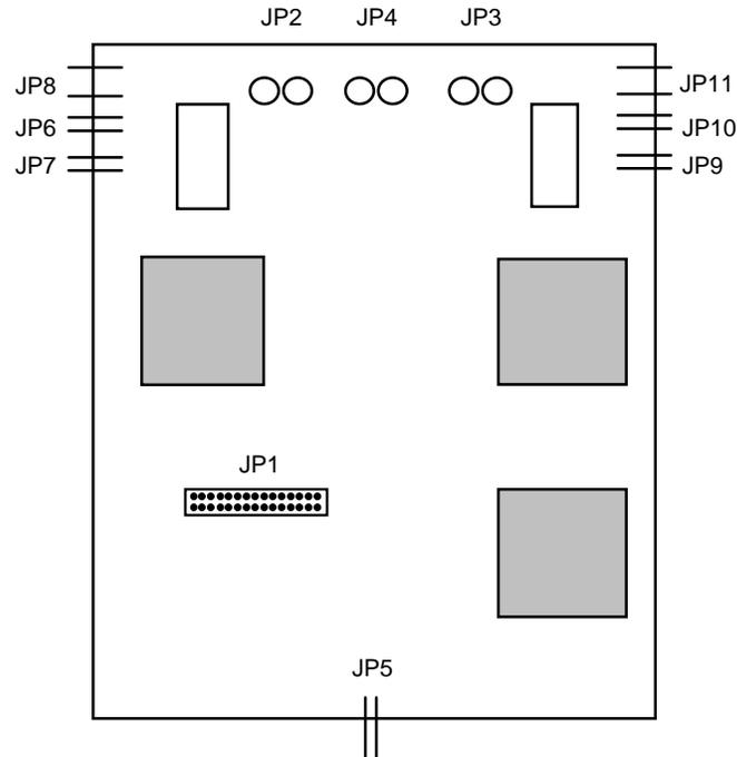
**Figure 5-1. Jumper Arrangements for the T1/E1 External Sync Panel**
