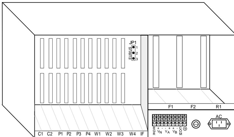
**Figure 1-2. Front-Loading Chassis (six-digit) with Power Supplies on Side**
