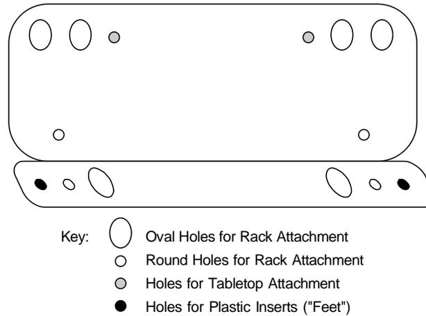
**Figure 2-2. Mounting Bracket Holes**
