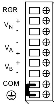
**Figure 2-11. Ground Connections (Front-Loading Chassis with Power Supplies on Top)**
