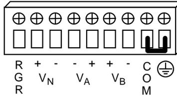
**Figure 2-10. Ground Connections (Two-Sided Chassis with Power Supplies on Side)**
