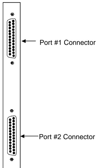
**Figure C-21. Two-Port HSU 530/35 Front Panel Connectors**
