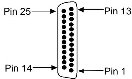
**Figure C-22. Two-Port HSU 530/35 Jack Pin Orientation**
