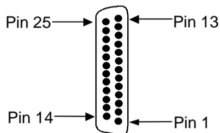
**Figure C-29. HSU-T V35 Card Jack Pin Orientation**
