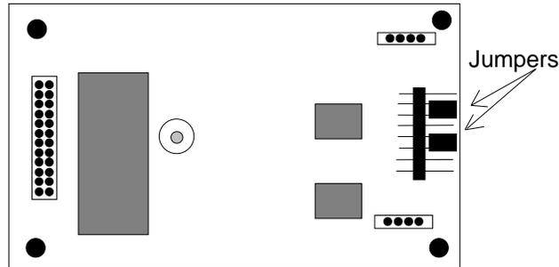
Figure 6-8. DSX/CEPT Revision E+ Module Jumpers
