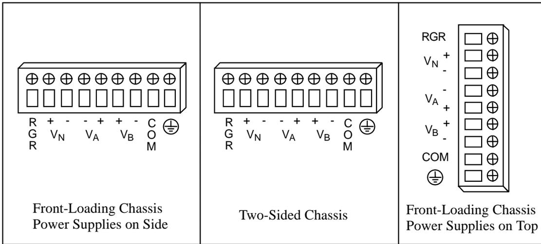
**Key:** ⊕ = Chassis Ground      COM = Common System Ground
