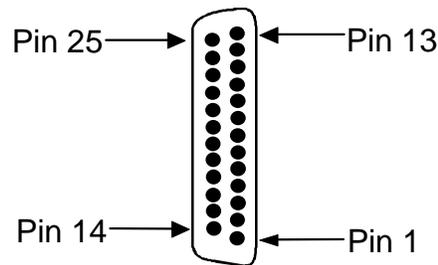
**Figure C-24. HSU 35 Card Jack Pin Orientation**
