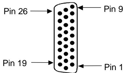
**Figure C-26. HSU-AD 530/35 Card Jack Pin Orientation**
