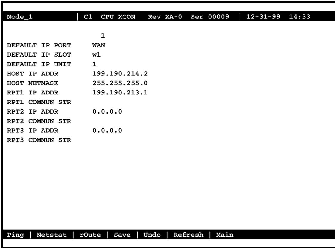
Figure 4-6. Typical TCP/IP Screen
