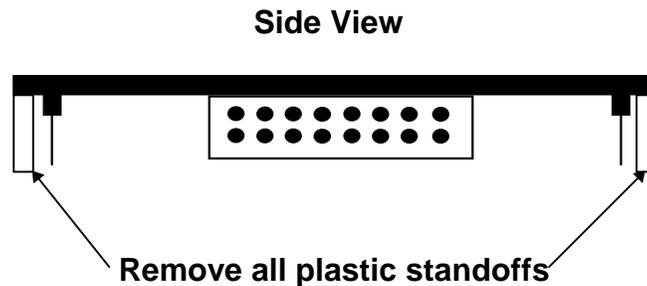
**Figure 6-18. Removal of Plastic Standoffs - 811 WAN Module**
