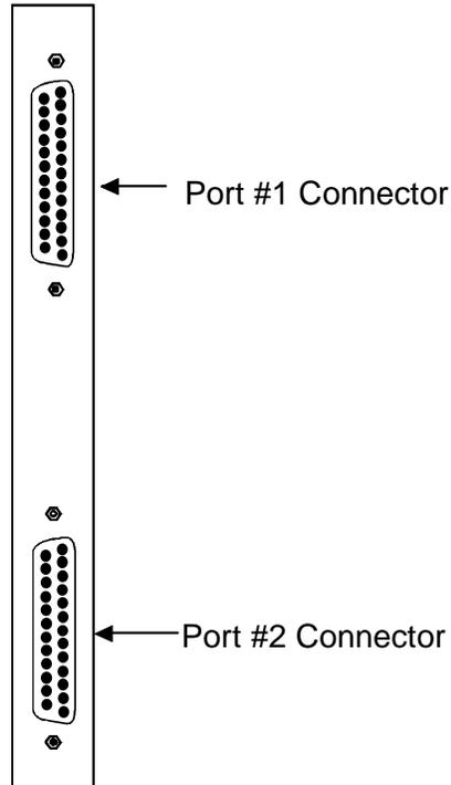
**Figure C-28. HSU-T V35 Card Front Panel Connectors**
