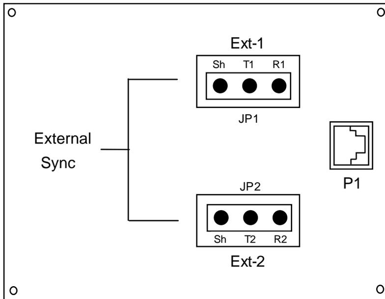
Figure 5-3. External Timing Sync Connection
