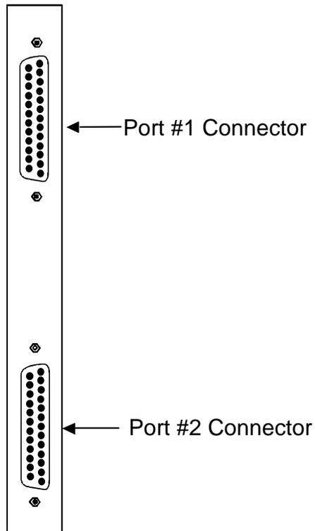
**Figure C-23. HSU-T V11 Card Front Panel Connectors**
