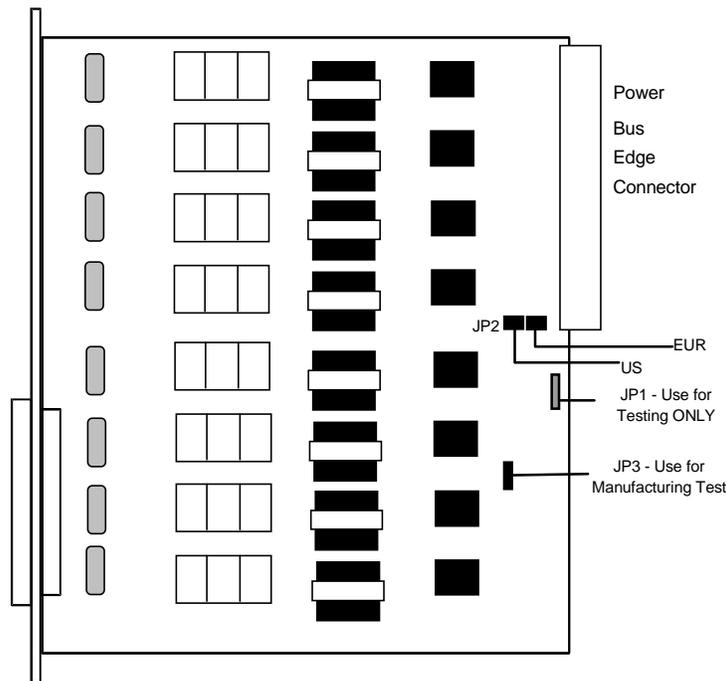
**Figure 6-1. P-Phone PPO and PPS Cards Jumper Settings**
