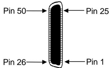
**Figure 6-2. P-Phone PPO and PPS Card Tip/Ring Connector**
