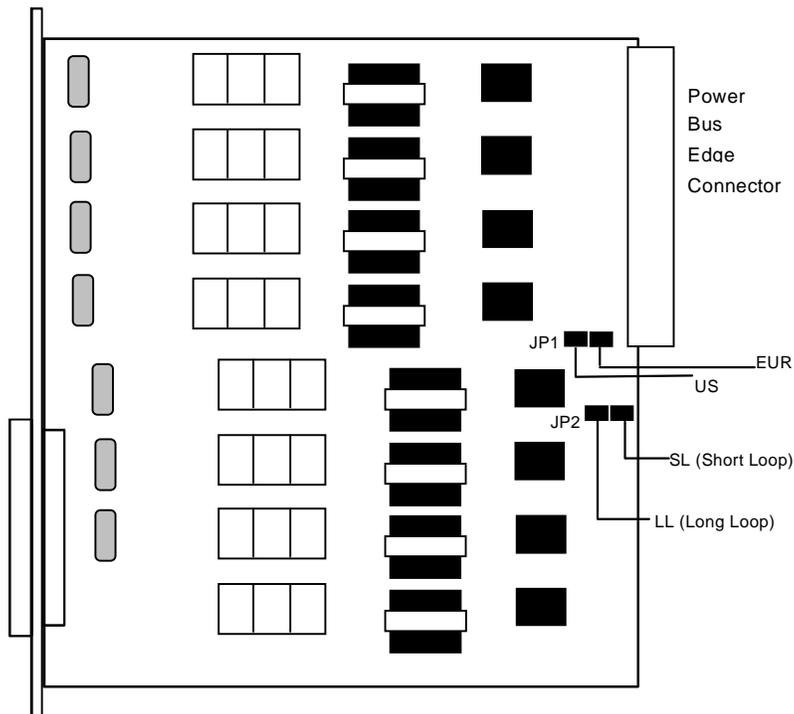
Figure 2-2. FXS 2W\*8-6 Card Jumpers Settings
