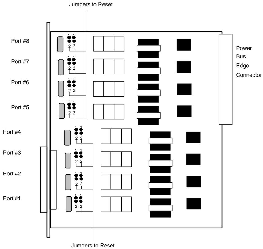
Figure 5-1. Jumpers for MRD Mode
