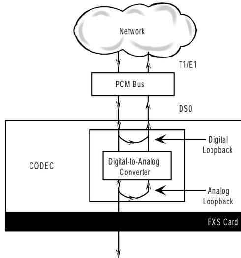
**Figure 2-4. FXS Card Loopbacks**
