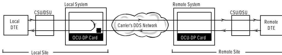
Figure 3-6. OCU Local Loopback (dte option)
