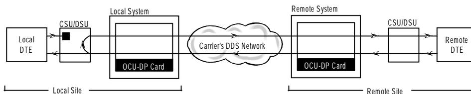
**Figure 3-11. OCU Remote Loopback (csu-u option)**
